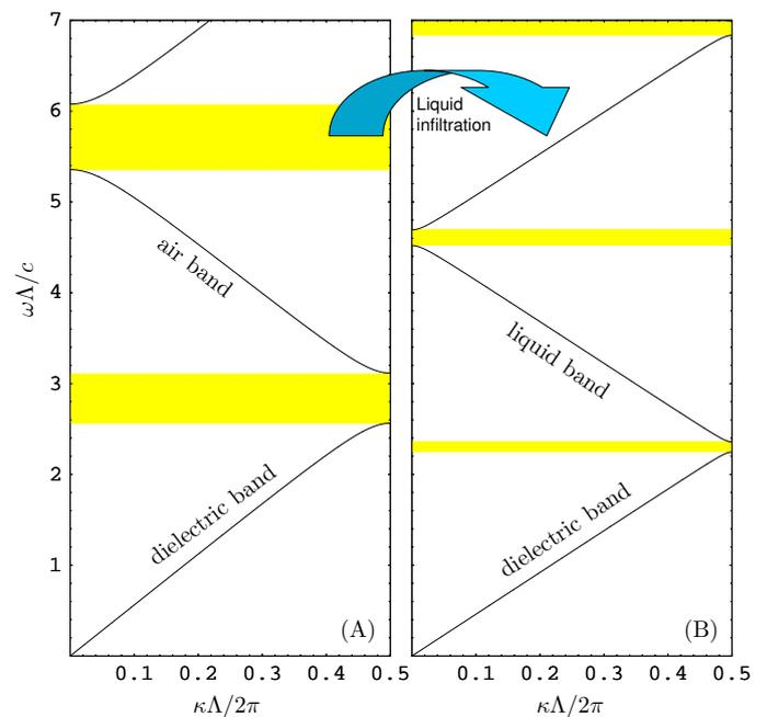
FIG. 2 (A) Band diagram for a Bragg stack with  $n_l = 1$  (corresponding to air),  $n_s = 1.5$  (corresponding to a typical polymer),  $b_l = 0.8\Lambda$ , and  $b_s = 0.2\Lambda$ . (B) Band diagram for the structure in (A), but with the air regions infiltrated by a liquid with  $n_l = 1.33$ .
