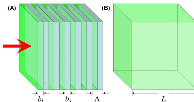
FIG. 1 (A) Liquid-infiltrated Bragg stack composed of alternating solid and liquid layers of thickness  $b_s$  and  $b_l$ , respectively. (B) Schematic illustration of a corresponding classical Beer-Lambert absorbance cell where the incident light passes through a spatially homogeneous medium, i.e. the liquid sample to be analyzed.
