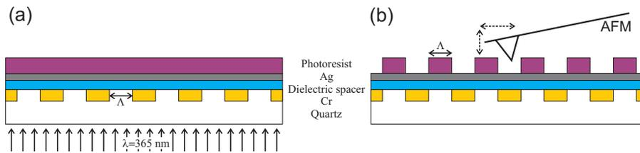
Fig. 1. Near-field superlens design using UV-lithography readout. (a) Exposure of negative photoresist through the quartz/Cr mask and the Ag superlens of a grating pattern with period  $2\Lambda$ . (b) AFM scan of the exposed and developed photoresist.
