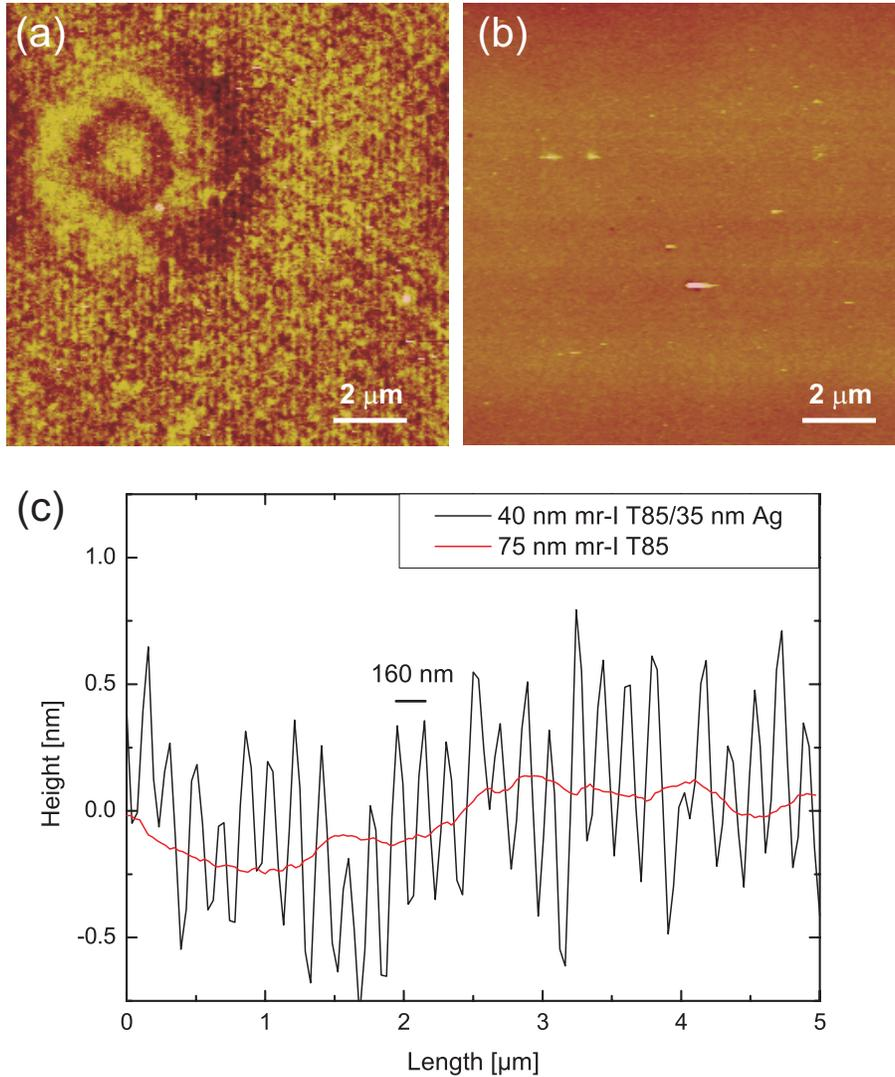
Fig. 7. (a)  $8 \times 8 \mu\text{m}$  AFM scan of the recorded image of 80 nm half-pitch gratings in the mr-UVL 6000 resist. The exposure was done through the Ag superlens. (b)  $8 \times 8 \mu\text{m}$  AFM scan of the obtained image of 80 nm half-pitch gratings in the resist where the Ag layer was replaced with mr-I T85. (c) Height scan of the images (a) and (b).
