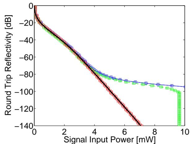
Fig. 4. The threshold for the distributed Raman amplified scheme, shown in Fig. 3, which is numerically calculated in the three cases of i) propagation including depletion, the thin blue solid line, ii) propagation without depletion on the Raman wave, the thin green dashed line, and iii) propagation without depletion on the Raman wave nor the signal wave, thin red dash dotted line, all with error bars. The thick black solid line show the derived threshold.
