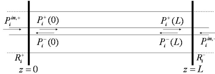
Fig. 1. A fiber cavity of length  $L$  with power reflectivity  $R_i^+$  in the left end and  $R_i^-$  in the right end creates a cavity. A CW input signal in this produce a Brillouin wave in the opposite direction. Both waves are amplified by a Raman amplifier. The signal output power, given by  $P_S^{\text{out}}(t) = (1 - R_S^-)P_S^+(L, t)$ , oscillates in case of high signal input power levels.
