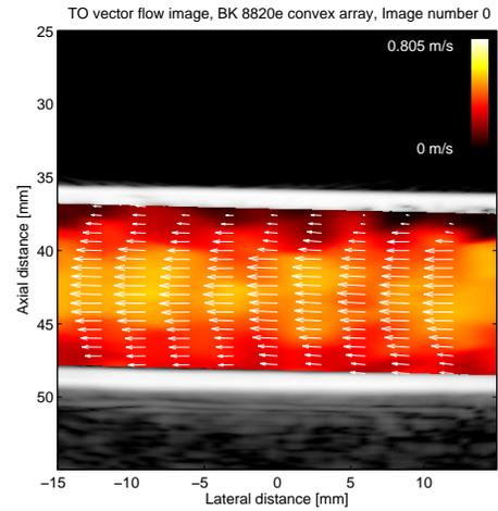
Fig. 8. Vector flow image measured on a flow rig phantom with a parabolic velocity profile and using the BK8820e convex array probe and the SARUS scanner.
