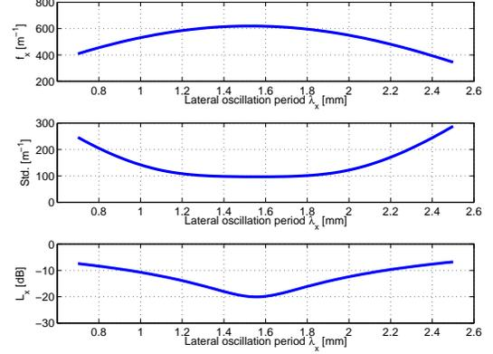
Fig. 2. Influence of a variation in the desired lateral oscillation period. The top graphs shows the obtained mean frequency, the middle graph the standard deviation of the field, and the lower graph the spectral leakage ratio.
