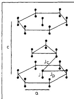
**Figure 1.** Schematic structure of  $\text{Cs}_3\text{Cr}_2\text{Cl}_9$  indicating the three exchange parameters. The hexagonal lattice constants are  $a = 7.14 \text{ \AA}$  and  $c = 17.72 \text{ \AA}$  at 2 K. Only the  $\text{Cr}^{3+}$  ions are shown.
