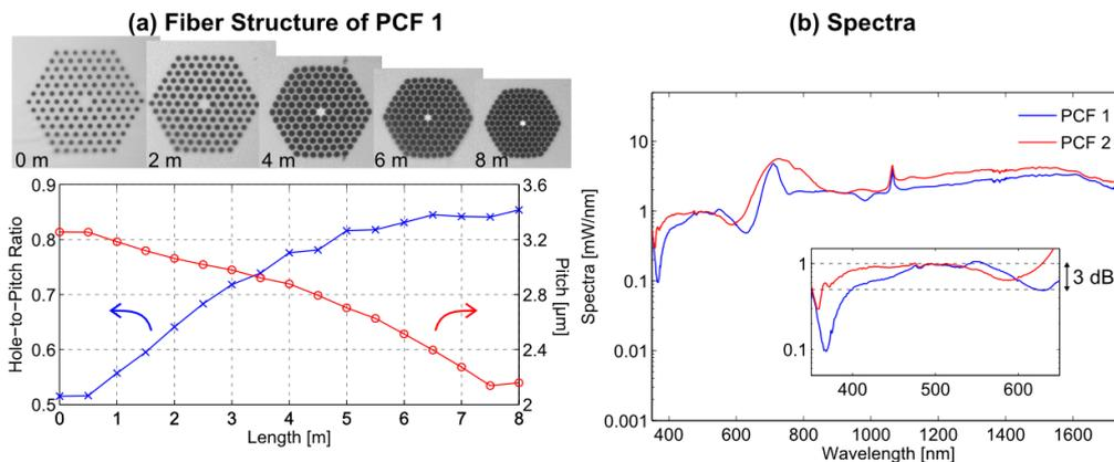
**Fig. 1** (a) Characterisation of the fiber structure of PCF 1. The top row shows microscope images of the fiber structure and the plot shows the corresponding hole-to-pitch ratio and pitch as a function of length. (b) Spectra of PCF 1 and 2. The inset shows a close up of the spectral blue edge and the 3 dB bandwidth of PCF 2. The fibers were pumped at 1064 nm with 10 ps pulses at 15 W average power and 80 MHz repetition rate.
