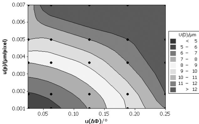
Figure 2: Contour plot of the expanded uncertainty of the diameter  $U(D)$  as a function of uncertainty values of pixel size  $u(p)$  and rotational angle  $u(\Delta\Phi)$ . The dots correspond to values of  $U(D)$  calculated in terms of the regression equation [4].
