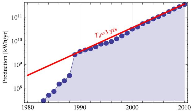
**Figure 1.** The global yearly production of electrical energy by wind turbines showing an exponential development over the last two decades with a doubling time of three years. Source: US Energy Information Administration.
