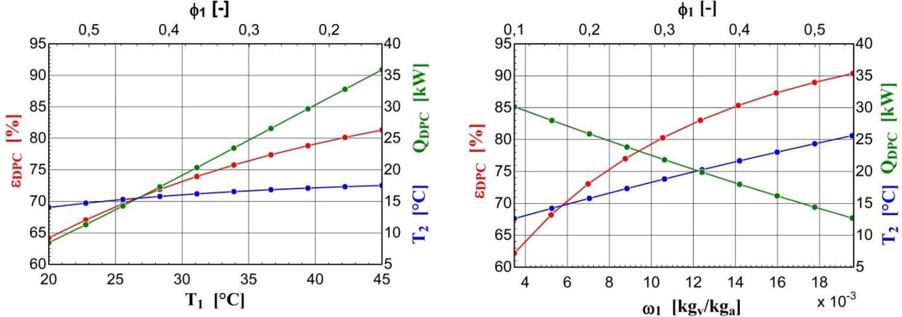
a) Constant inlet humidity ratio ( $\omega_1=8$  [g<sub>v</sub>/kg<sub>a</sub>])b) Constant inlet temperature ( $T_1=35$  [°C])Figure 6. Analysis on primary inlet thermo-hygrometric conditions ( $\dot{V}_1=4200$  [m<sup>3</sup>/h],  $f_{rec}=0.3$ )
