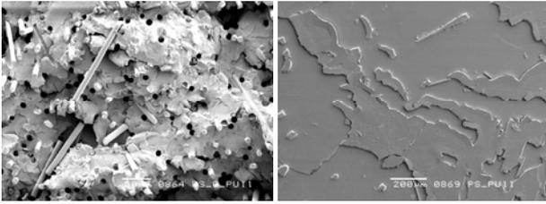
Figure 5: Broken surface of PS molded tensile bar after tensile testing (left hand side picture- taken on the sample with glass and right hand side picture -taken on the samples without glass).
