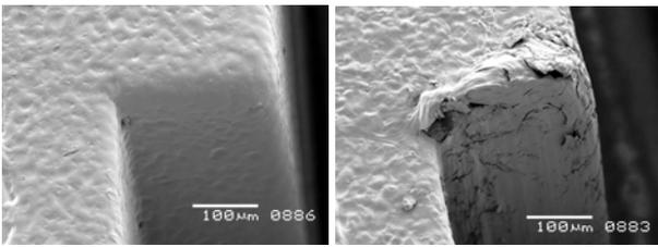
Figure 6: Effects of glass fibers on micro cracks of the injection molded plastic parts (Part without glass fiber-left picture, part with glass fiber-right picture).
