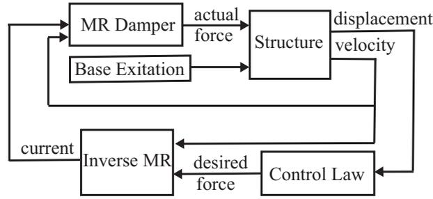
Figure 9: Schematic diagram for closed loop simulation
