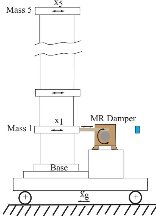
Figure 1: Shear Frame Structure with MR damper
