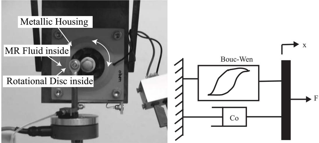
Figure 2: Rotational MR Damper and Bouc-Wen damper model
