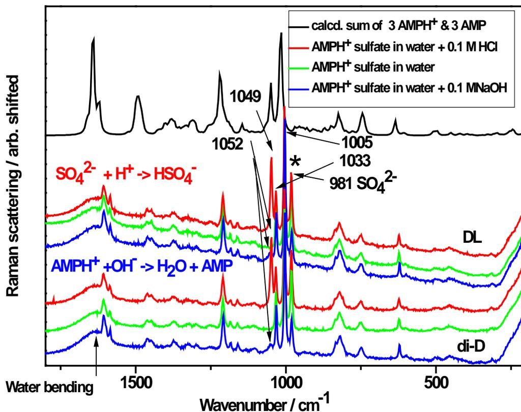
**FIG. 6.** Raman spectra of 30 mg/mL aqueous solutions of DL- and di-D-amphetammonium sulfate, ca. 30.4 mg in 1 mL water obtained at 25 °C with 514.5 nm laser light, 11 mW through a 10X objective, on the LABRAM instrument. Acquisition time was 1x20 sec. For comparison, the sum of all six calculated AMP and AMPH<sup>+</sup> model spectra is included. An asterisk is labelling the SO<sub>4</sub><sup>2-</sup> sym stretching. To make the solutions acidic or basic 0.1M HCl or NaOH was used.
