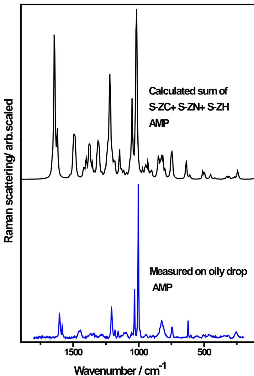
**Fig. 9.** Raman spectrum from an oily droplet separated from a DL-AMPH<sup>+</sup> sulfate solution to which enough NaOH has been added. The spectrum shows that the oil consisted of AMP. The sum of the three calculated AMP conformations is given for comparison. Experimental Conditions: LABRAM instrument with 514.5 nm laser light, 11 mW through a 10X objective, neutral density filter half open, hole 600 nm, slits 100 nm, acquisition time 6x10 sec.
