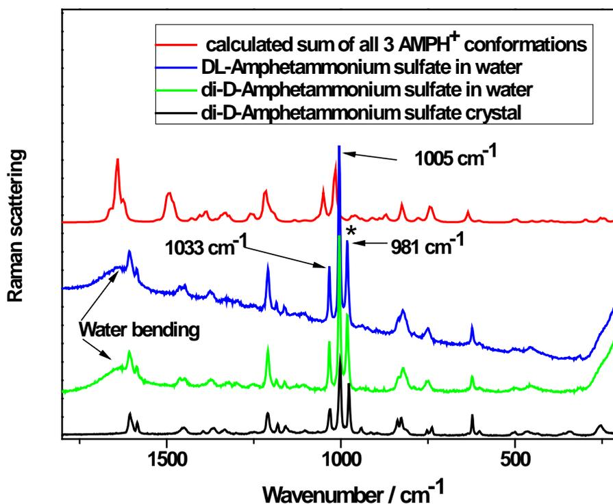
**Fig. 5.** Comparison of Raman spectra of solid di-D- and aqueous solutions (ca. 0.08 mol/L in water), of DL- and di-D-amphetammonium sulfate obtained at 25 °C on the LABRAM Raman instrument and with 514.5 nm laser light, 11 mW through a 10X objective. Acquisition time for the solutions 1x20 sec, for the solid 1x10 sec. For comparison a sum of calculated AMPH<sup>+</sup> model spectra is shown. The asterisk is labelling the SO<sub>4</sub><sup>2-</sup> sym stretching.
