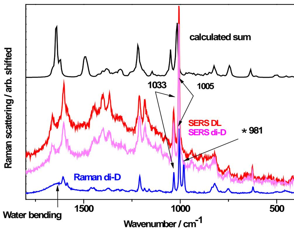
**Fig. 11.** SERS spectra obtained of DL-AMPH<sup>+</sup> sulfate and di-D-AMPH<sup>+</sup> sulfate in dilute solutions (concentrations of 2.6 mM AMPH<sup>+</sup>). Conditions: LABRAM, 514.5 nm excitation, 11 mW through a 10X objective, acquisition times 1 x 10 sec. For reference the calculated sum of the three AMPH<sup>+</sup> conformations is shown at the top and the normal Raman spectrum of a 0.08 M (AMPH)<sub>2</sub>SO<sub>4</sub> solution at the bottom.
