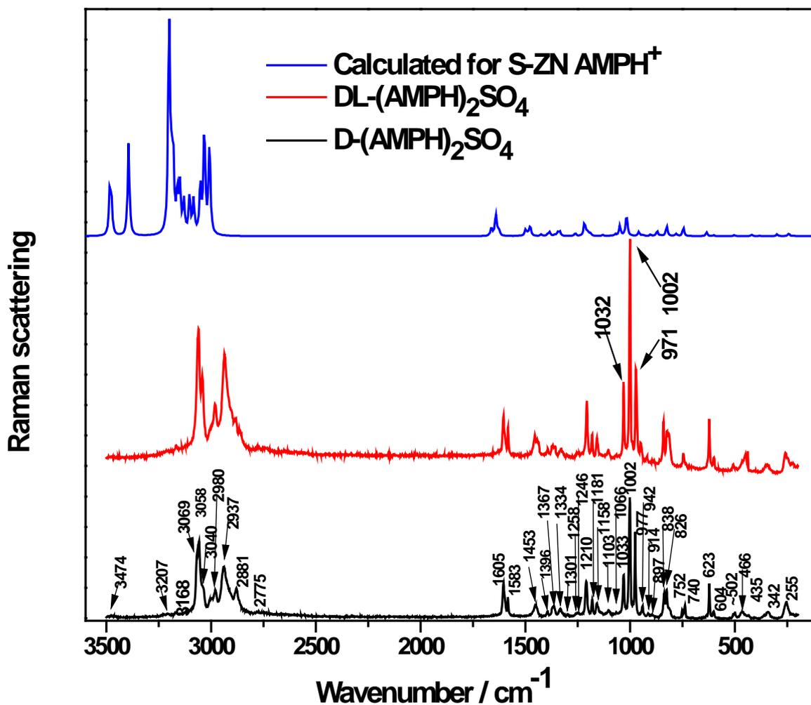
**Fig. 4.** Raman spectra of solid DL- and di-D-amphetammonium sulfates, obtained on the LABRAM instrument with 514.5 nm laser light, 11 mW through a 10X objective, acquisition times being 1x10 sec. For comparison the calculated spectrum for the AMPH<sup>+</sup> ion in S-ZN conformation is shown.
