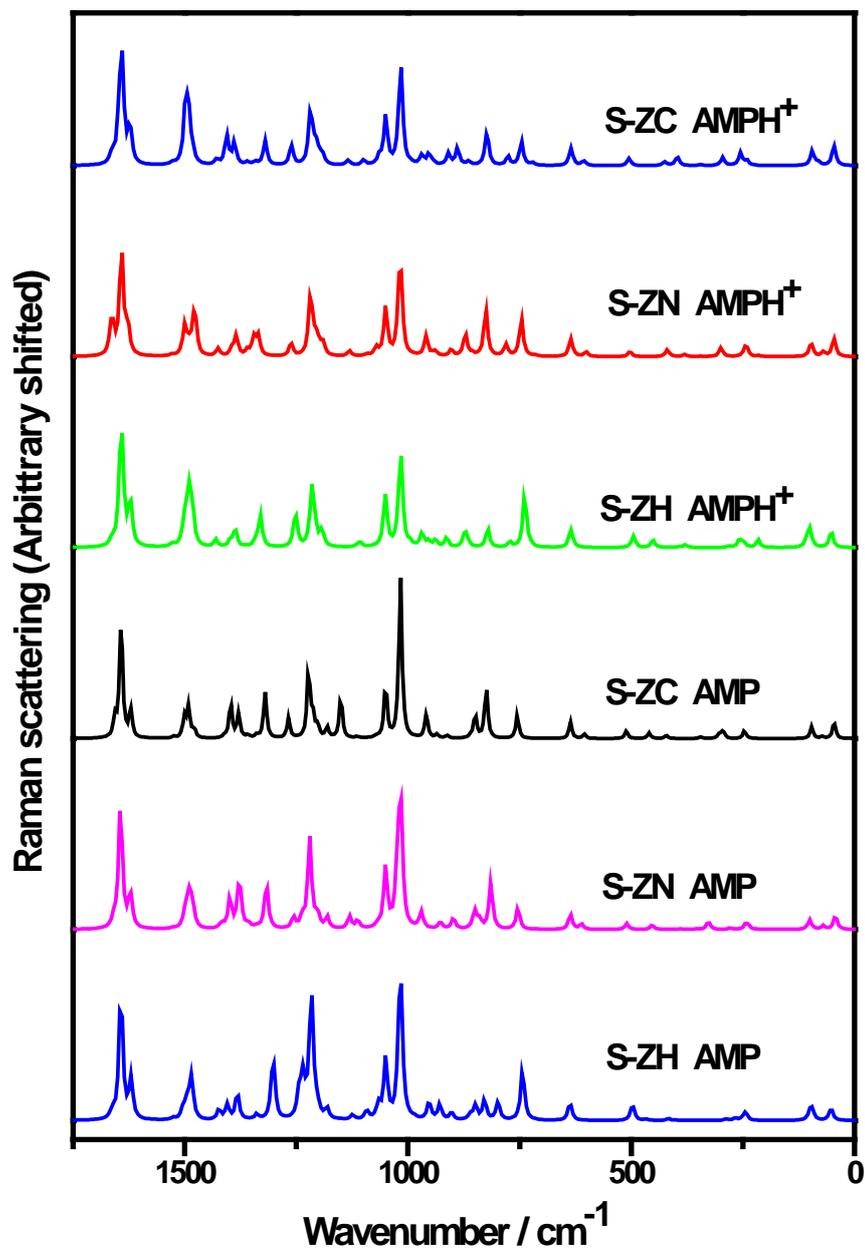
**FIG. 3.** Calculated Raman spectra in the low wavenumber-range (1750-0 cm<sup>-1</sup>) of the S-amphetamine-H<sup>+</sup> ion and the S-amphetamine molecule in their three different conformational geometries S-ZC, S-ZN and S-ZH.
