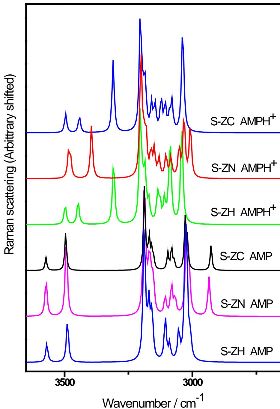
**FIG. 2.** Calculated Raman spectra in the high wavenumber-range (3650-2650 cm<sup>-1</sup>) of the S-amphetamine-H<sup>+</sup> ion and the S-amphetamine molecule in their three different conformational geometries S-ZC, S-ZN and S-ZH.
