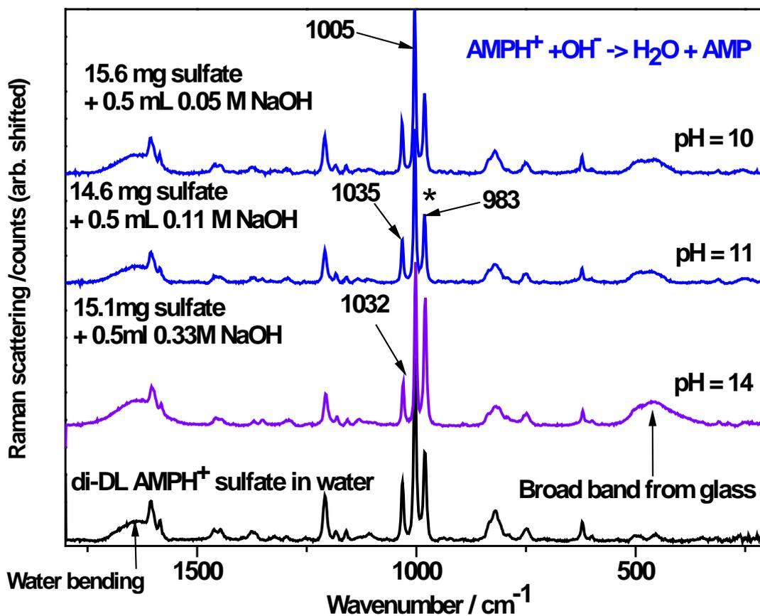
FIG. 7. Raman spectra versus the relative amounts of DL- $\text{AMPH}^+$  sulfate and NaOH in aqueous solutions. The pH acidity is given. Raman conditions: LABRAM, 514.5 nm, 11 mW through a 10X objective, neutral density filter fully open, hole 600, slits 100, 6x30 sec.
