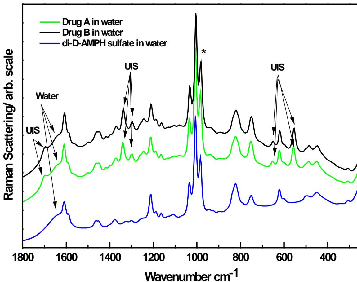
**FIG. 10.** Raman spectra of solutions of street drug powders, dissolved in water and filtered. Drug A solution is of a concentration of 60 mg/mL, drug B of 64 mg/mL. Also shown is the spectrum of di-D-amphetammonium sulfate at a concentration of  $\approx 0.08$  M  $(AM\ PH)_2SO_4$ , or 0.16 M  $AMPH^+$ . UIS = Unidentified substance. The sulfate stretching band is indicated with an asterisk.
