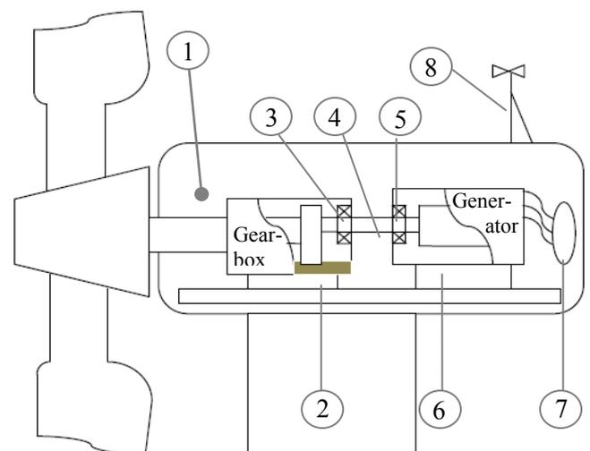
Figure 1: Schematic of sensors in a wind turbine [6]
