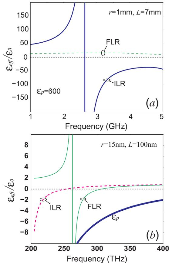
**Figure 2.** Effective permittivity  $\epsilon_{\text{eff}}$  for a rod-type MM with a cubic unit-cell. (a) Dielectric rods with  $\epsilon_p = 600$ ,  $r = 1$  mm and  $L = 7$  mm with the results contrasting infinitely long rods (ILR) with finite-length rods (FLR) ( $l = 6.95$  mm). (b) Rods supporting a dispersive plasma with  $r = 15$  nm and  $L = 100$  nm with the results contrasting ILR with FLR ( $l = 80$  nm).
