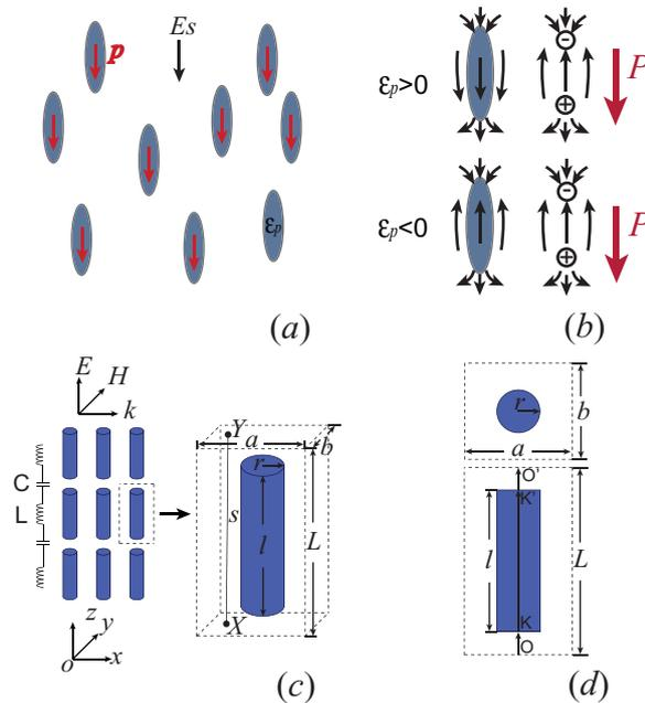
**Figure 1.** (a) Dilute mixture of sub-wavelength particles. The red arrows indicate the direction of polarization. (b) Schematics of polarization, contrasting different signs of permittivity. The black arrows represent the  $E$ -field direction.  $\epsilon_p = \epsilon'_p + i\epsilon''_p$  is the relative dielectric constant of the particle. (c) Schematic diagram of rod-type MM and the corresponding equivalent circuit model. (d) Top and side views of a single unit-cell.
