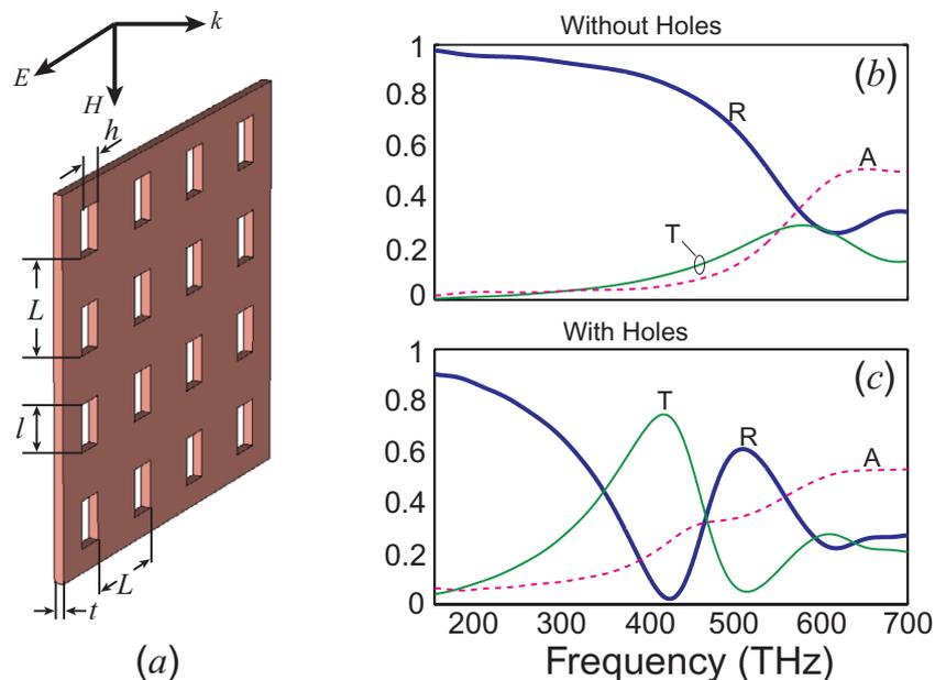
**Figure 4.** (a) Gold thin film with  $t = 30$  nm,  $l = 75$  nm,  $h = 12$  nm and  $L = 100$  nm. (b) Full-wave simulations of the EM response in the absence of any holes. (c) The corresponding response in the presence of an air-hole array. Still, in the simulation there is one unit-cell in the  $\hat{k}$ -direction and periodic boundary condition applied in the in-plane directions. The unit-cell length in the  $\hat{k}$ -direction is  $L$ .
