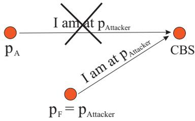
Fig. 3. Position spoofing attack. Attacker spoofs node  $A$  and CBS into believing that it (the node) is at its (attacker’s) position  $p_F$ . The attacker then replays node’s message from  $p_F$  to fool the position verification mechanism.
