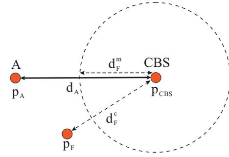
Fig. 2. False position report by node  $A$  to the covert base station.  $p_A$  is the true node position,  $p_F$  is the fake node position (reported by  $A$  to CBS),  $p_{CBS}$  is the position of CBS.  $d_F^c = d(p_F, p_{CBS})$  is the (false) distance between CBS and  $A$ , computed by CBS,  $d_F^m$  is the (false) distance between  $A$  to CBS measured passively by CBS. If  $|d_F^c - d_F^m| \leq \Delta$ , then  $p_A = p_F$ .
