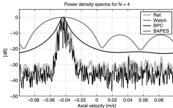
Fig. 2. The mean of the PSD estimates for  $N = 4$ ,  $L = 400$  and  $K = 40$ . The reference PSD is given in light gray. Welch's method fails miserably in finding the PSD. Also the BPC displays one sharp peak instead of the true distribution. Only the BAPES can be considered to resolve the PSD as well as the reference.
