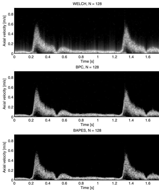
Fig. 4. The spectrogram for the three methods when  $N = 128$  with a dynamic range of 40 dB. All three methods are able to properly show the spectrogram. The sidelobes visible in the Welch spectrogram are a result of the rectangular weighting of the data. These could easily be removed using another weighting at the expense of spectral resolution.
