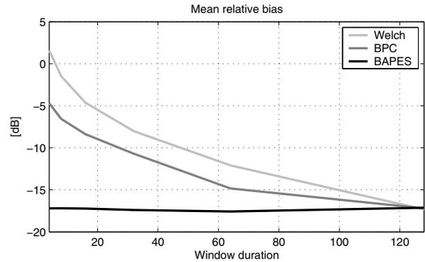
Fig. 3. The MRB for the three methods. BAPES shows the best performance and is not improved as  $N$  grows. The BPC is better than Welch's method and improves in terms of MRB as  $N$  grows.
