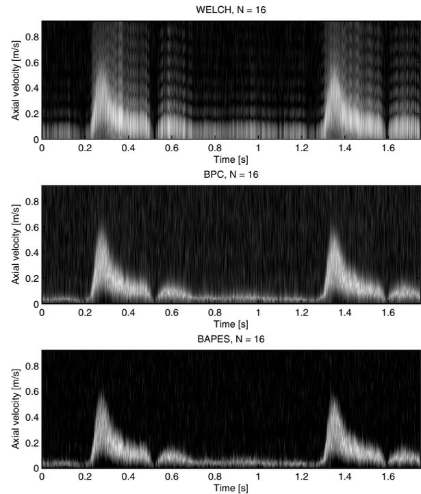
Fig. 5. The spectrogram for the three methods when  $N = 16$  with a dynamic range of 40 dB. The spectral resolution of Welch's methods is here much too poor to reproduce the spectrogram correctly. The BPC has sufficient spectral resolution and so has BAPES. BAPES displays slightly better signal to noise ratio than the BPC.
