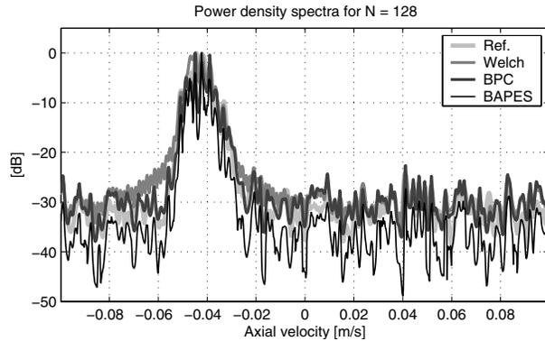
Fig. 1. The mean of the PSD estimates for  $N = 128$ ,  $L = 400$  and  $K = 40$ . The reference PSD is given in light gray. All three methods are able to resolve the spectrum of the blood signal. Welch's method displays more spectral smoothing compared to BPC and BAPES.
