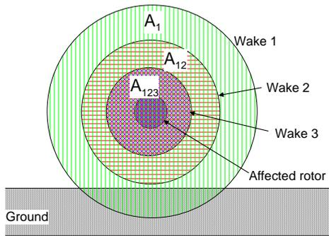
Figure 13 Tiles in wake for straight row of wind turbines in line with wind direction.
