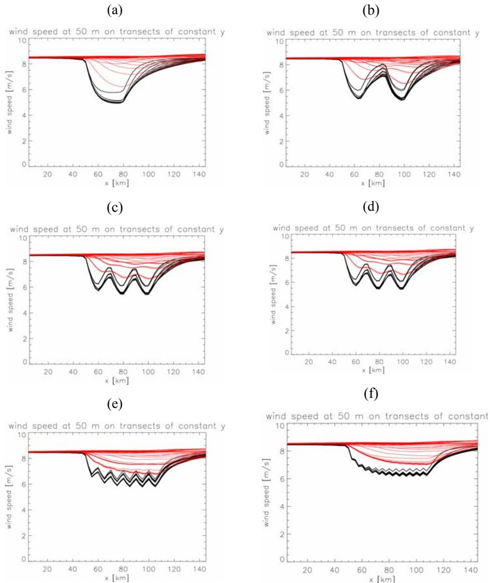
Figure 22. Plots showing transects along constant northing of the mean wind speed calculated for 3 simulations in the westerly sector, for each of the 6 wind farm configurations listed in the table: Exp ID 1, (a), 2, (b), 3 (c), 4, (d), 5, (e), 6, (f). Black and red lines show transects that do pass and transects that do not pass through the wind farm grid cells respectively.
