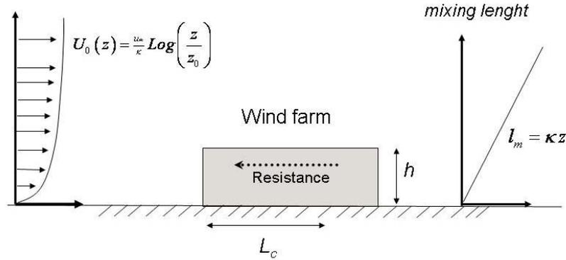
Figure 18 *Illustration of the model setup with a incoming windprofile and a wind farm which acts with a force on the incoming flow the height  $h$  is considerably higher than the roughness and therefore the modeling of the flow through the wind farm has to be established to predict how the flow behind the wind farm behaves.*
