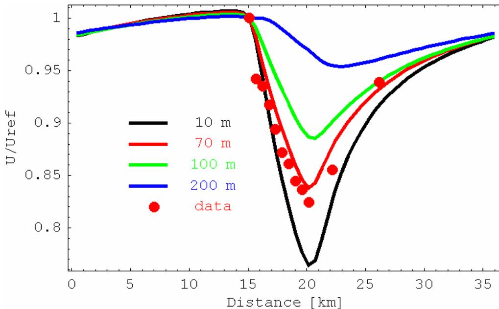
Figure 20. Normalized wind speed through the wind farm and behind the wind farm compared to measurements at Horns rev.
