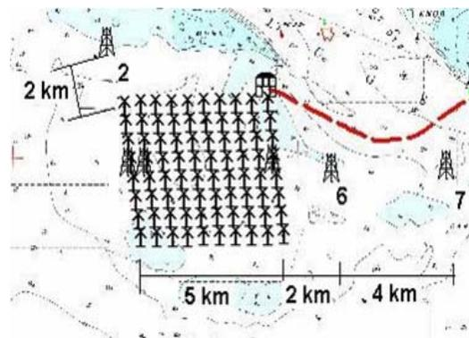
Figure 2 The position of the meteorological towers. The “downwind” met masts are off-line relative to the West-East wind turbine rows – placed on a line in the middle of two rows.
