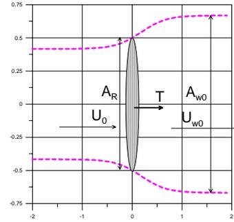
Figure 12. Near range flow around the rotor.
