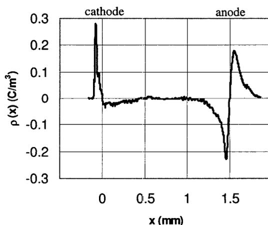
Fig. 3. Steady state space charge distribution obtained after poling but with a temperature gradient. The cathode and anode temperatures were 70°C and 43°C respectively. Electrodes were grounded during measurement.
