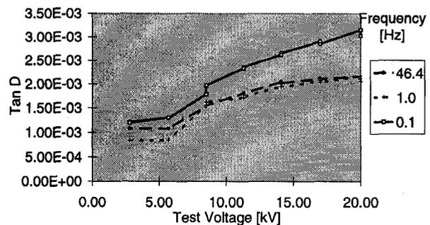
Fig. 7:  $\tan\delta$  measured at 46, 1, 0.1 Hz by dielectric spectroscopy
