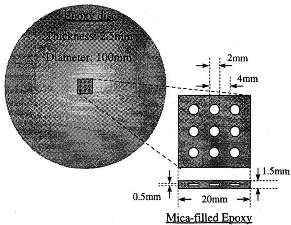
Fig. 2: Test sample with 9 cylindrical voids
