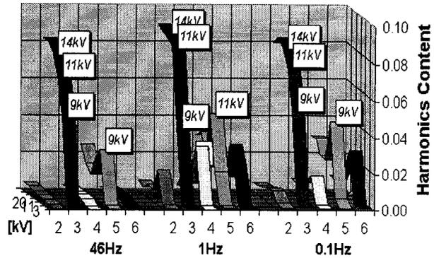
**Fig.10:** Content of harmonics (2<sup>nd</sup>-6<sup>th</sup>) in the current through the test object at 46, 1, 0.1 Hz.
