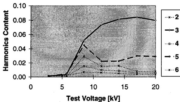
**Fig.9:** Content of harmonics (2<sup>nd</sup>-6<sup>th</sup>) in the current through the test object at 0.1 Hz.
