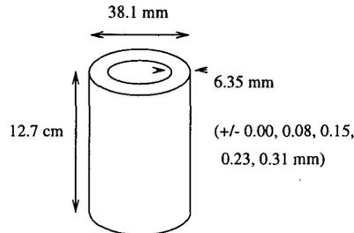
Figure 1: Schematic of the standard and comparison cylinders.
