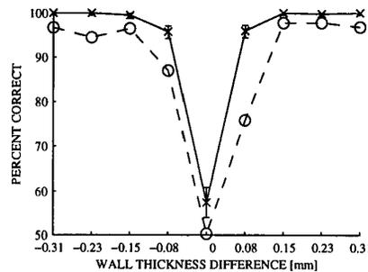
Figure 7: Results from artificial experiment (x-markers connected with full line including 90%-confidence intervals) compared with results from a similar experiment involving a false killer whale (o-markers connected with dashed line).
