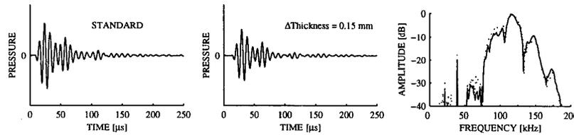
Figure 4: Echoes from the standard and the comparison cylinder that was 0.15 mm thicker than the standard cylinder. The waveforms are shown in the first two plots and the frequency spectra in the last plot. In the spectral plot the solid line is for the standard and the dotted line is for the comparison target.
