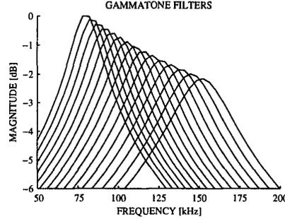
Figure 5: Frequency response for the gammatone filterbank.
