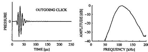
Figure 3: Waveform and spectrum of the projected simulated dolphin sonar signal.
