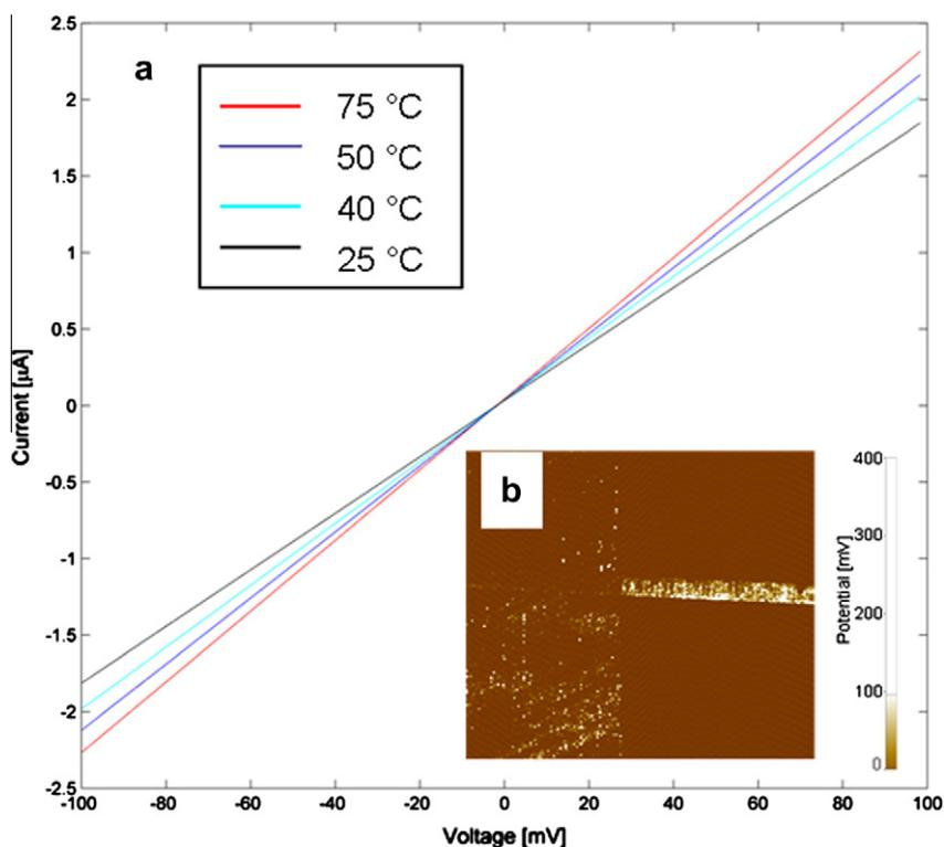
**Fig. 3.**  $I$ - $V$  curves for the nanowire devices at different temperatures is plotted to demonstrate the completely linear ohmic behavior of the PEDOT:TsO nanowire indicating a good contact between the gold electrodes and the PEDOT:TsO nanowire (a). In (b) an image acquired with conductive AFM is included to show the complete removal of the isolating peptide nanotubes from the surface of the PEDOT:TsO.
