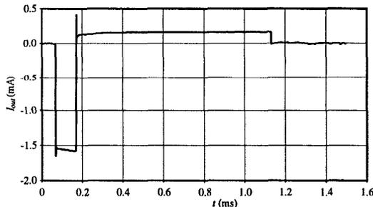
Figure 9. Measured output current pulse from the stimulator
