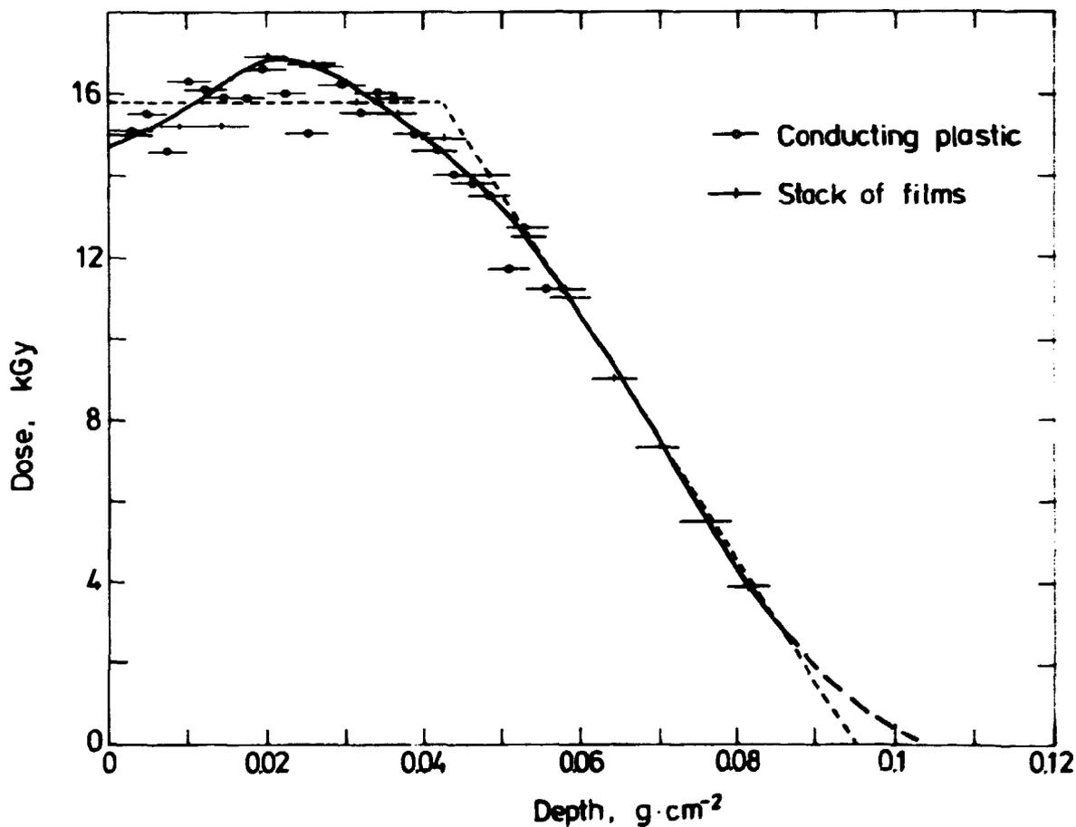
Fig. 13. Depth dose measurements at the 400 keV electron accelerator at Risø. One set of measurements were carried out with a stack of 50  $\mu$ m electrically isolating dosimeter films, while another set of measurements was made with dosimeter films at different depths of electrically conducting plastic.
