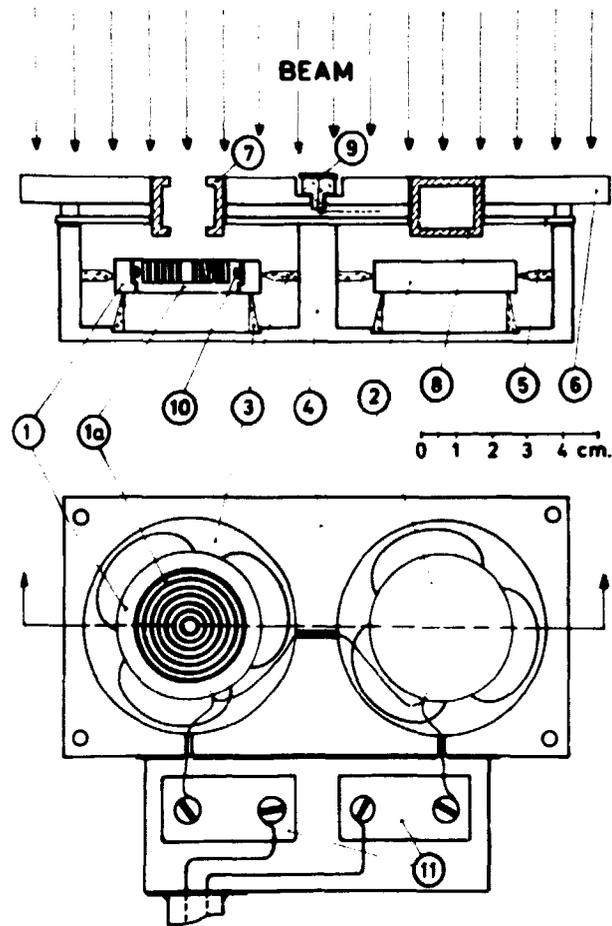
Fig. 14. Calorimeter for calibration of dosimeters irradiated at low energy electrons (Radak et al., 1973).
