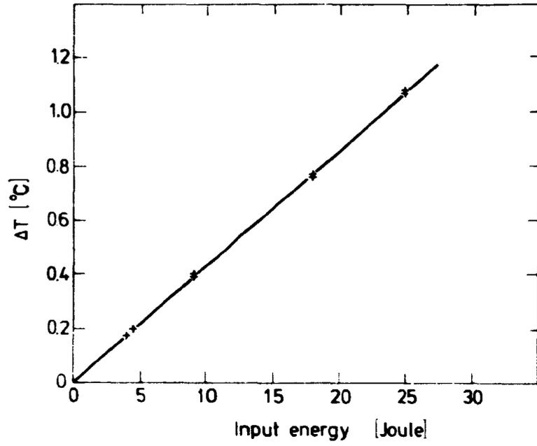
Fig. 15. Electrical calibration of the calorimeter of Fig. 14.
