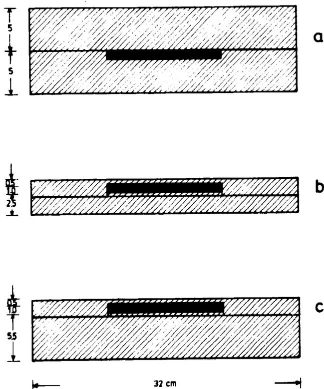
Fig. 12. Graphite calorimeters with different isolation configurations.
