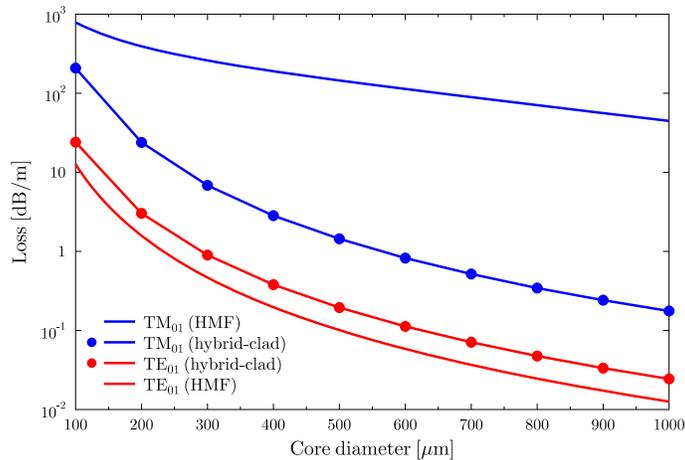
Fig. 8. Loss values for  $TE_{01}$  and  $TM_{01}$  modes guided by hybrid-clad fiber as a function of core diameter. The same curves for the full-metal fiber are also shown.  $\lambda = 10.6\mu\text{m}$ ,  $\Lambda = 2\mu\text{m}$ ,  $f_m = 0.2$ . The inner cladding has one layer of metal wires.
