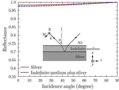
Fig. 3. Reflectance of TE-polarized incident light from two types of substrates, one plain silver and the other silver but with an indefinite medium layer on top (inset). The wavelength is  $10.6\mu\text{m}$ .
