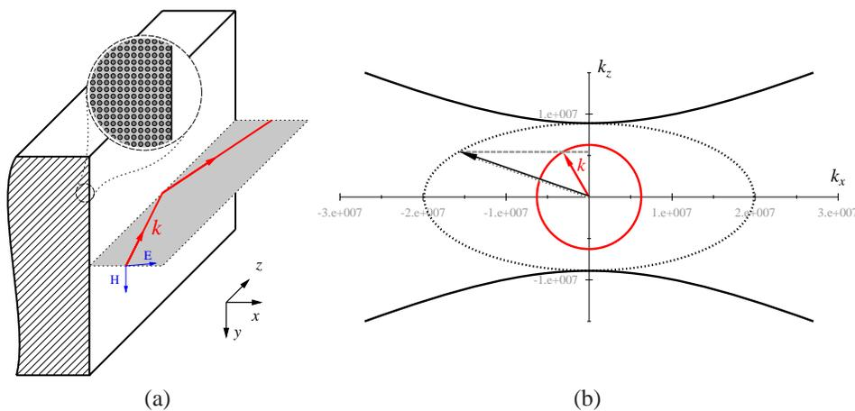
Fig. 1. (a) Metal-wire medium as a TM reflector in planar geometry. (b)  $k_x \sim k_z$  relations for TM light in both air (red curve) and an indefinite medium with  $\epsilon_x = 2, \mu_y = 1, \epsilon_z = -10$  (black curves), together with wavevectors illustrating reflection for TM light incidence. Axis unit: rad/m.  $\lambda = 1 \mu\text{m}$ .
