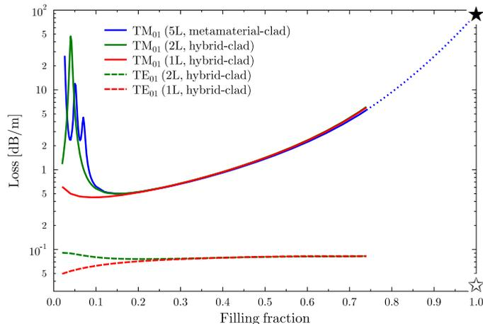
Fig. 7. Propagation losses of both  $TM_{01}$  and  $TE_{01}$  modes as a function of metal filling fraction.  $\lambda = 10.6\mu\text{m}$ ,  $\Lambda = 2\mu\text{m}$ . The propagation loss values for the  $TM_{01}$  and  $TE_{01}$  modes at the  $f_m = 1$  limit are marked as  $\star$  and  $\star$ , respectively.
