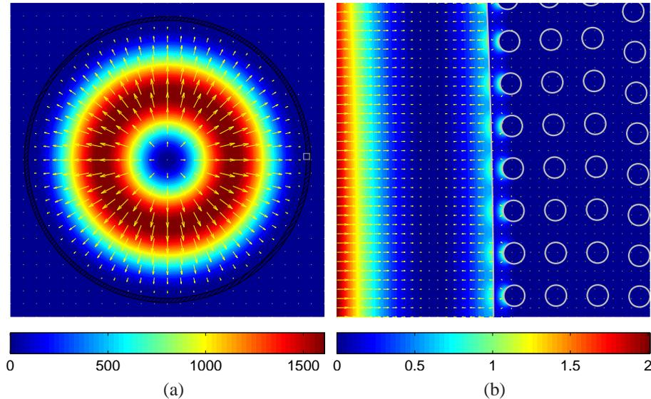
Fig. 6. Cross-sectional field distribution of the guided  $\text{TM}_{01}$  mode in a metamaterial-clad fiber with a  $700\mu\text{m}$  core diameter. (a) Overall mode; (b) The zoom-in plot of the region outlined in (a) by the gray line ( $15 \times 15\mu\text{m}^2$ ). Color shading is for the real part of the axial Poynting vector, while arrows are for transverse electric field.  $\lambda = 10.6\mu\text{m}$ ,  $\Lambda = 2\mu\text{m}$ ,  $f_m = 0.2$ .
