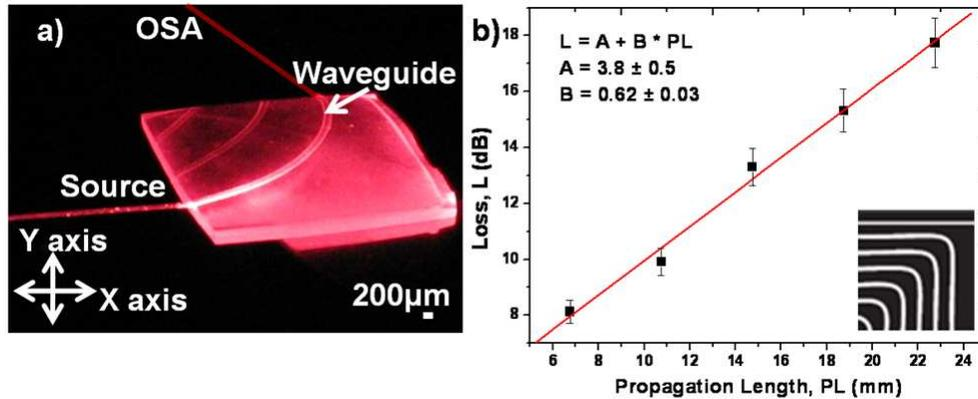
Fig. 2. (a) Experimental setup for measuring propagation and bend loss in the NP LCW, (b) Loss ( $L$ ) in waveguides with different lengths as a function of propagation length ( $PL$ ). The solid curve is a linear fit to the measured data. (Inset)  $1.5 \times 1.5$  cm UV mask designed for measuring propagation loss in NP polymer LCW.
