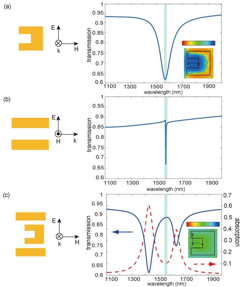
Fig. 2. Simulated transmission spectra of (a) SRR (b) paired rods (c) the combination of SRR and paired rods. The insets show  $H_z$  for SRRs at 1560nm.
