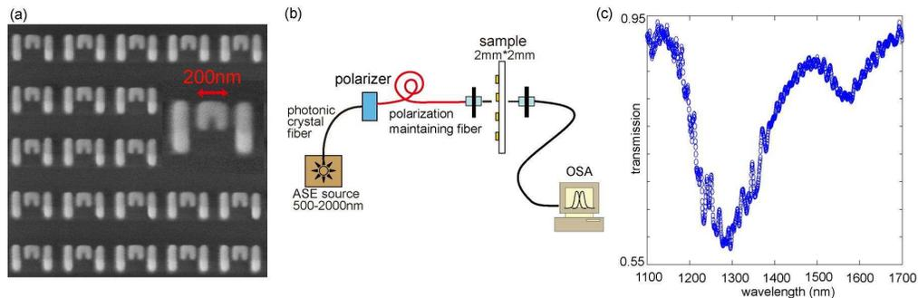
Fig. 3. Panel (a) shows a micrograph of a SRR array with pitch =  $800\text{ nm}$ . The inset gives an enlarged view of the structures. Panel (b) illustrates the measurement setup. Panel (c) shows the measured spectral transmission.
