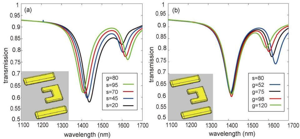
Fig. 5. Transmission spectra (a) for different lateral displacement  $s$  calculated at  $g = 80$ nm (b) for different gap  $g$  calculated at  $s = 80$ nm. The insets show the structure used in the simulation.
