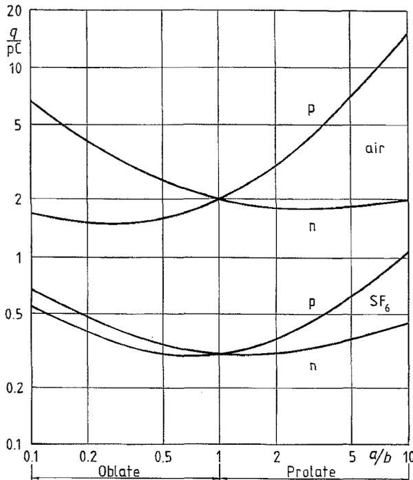
Figure 7. Poissonian induced charge  $q$  for spheroidal voids in a coaxial disc spacer. See text for conditions.  $p$ :  $E_0$  parallel to void axis of rotation.  $n$ :  $E_0$  normal to void axis of rotation.
