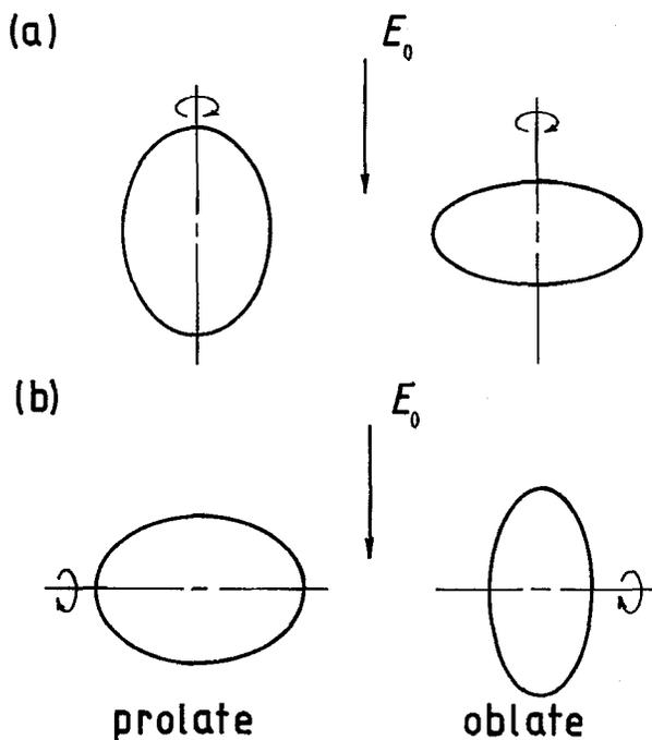
Figure 1. Void orientation with respect to the applied field  $E_0$ . (a)  $E_0$  parallel to void axis of rotation (b)  $E_0$  normal to void axis of rotation.
