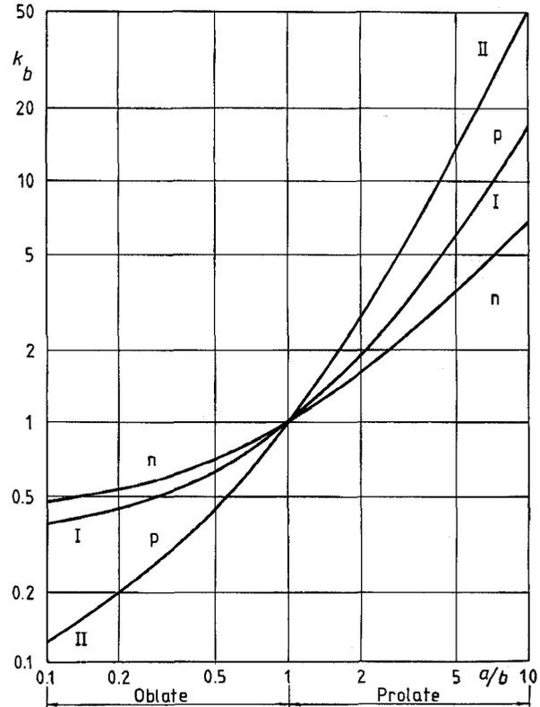
Figure 6. The shape factor  $k_b$  for spheroidal voids. I: strongly attaching gas, II: weakly or non-attaching gas.  $p$ :  $E_0$  parallel to void axis of rotation.  $n$ :  $E_0$  normal to void axis of rotation.
