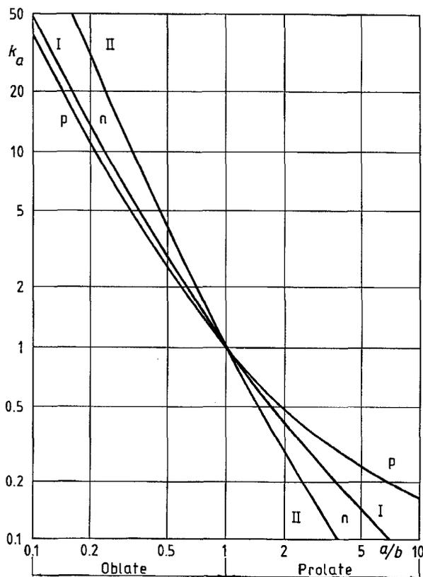
Figure 5. The shape factor  $k_a$  for spheroidal voids. I: strongly attaching gas, II: weakly or non-attaching gas.  $p$ :  $E_0$  parallel to void axis of rotation.  $n$ :  $E_0$  normal to void axis of rotation.
