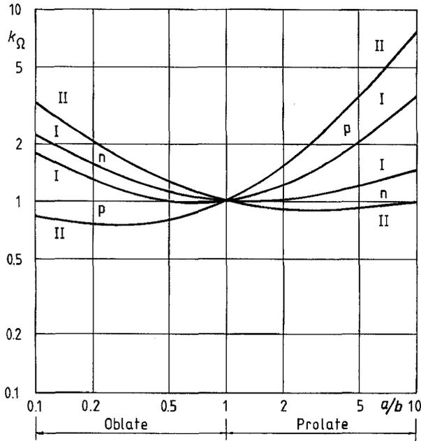
Figure 4. The shape factor  $k_{\Omega}$  for spheroidal voids. I: strongly attaching gas, II: weakly or non-attaching gas.  $p$ :  $E_0$  parallel to void axis of rotation.  $n$ :  $E_0$  normal to void axis of rotation.
