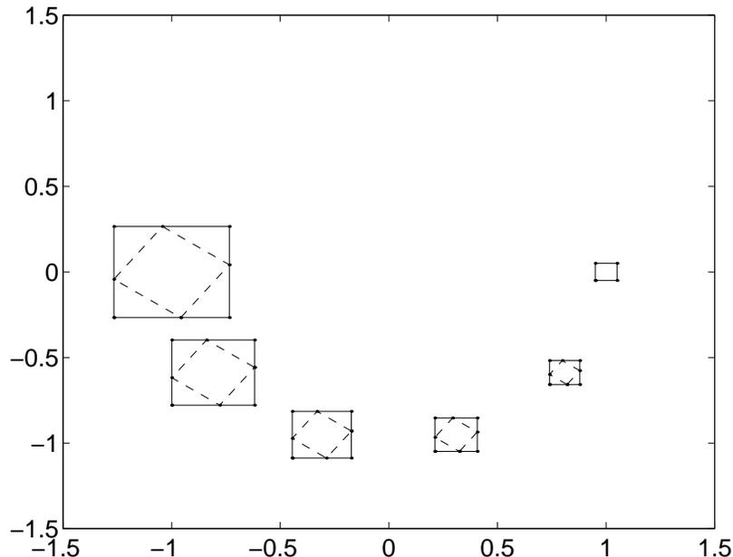
Figure 4.1: Five simple interval iterations, using the map in Eq. (4.3) with  $\Delta t = \frac{\pi}{5}$  and the initial interval vector  $([x_0], [y_0]) = ([0.95, 1.05], [-0.05, 0.05])$ . The solid rectangles are the interval vector enclosures  $\{([x_j], [y_j])\}_{j=0, \dots, 5}$  while the dashed rectangles are their images  $\mathcal{R}(\varphi_{rot}, ([x_j], [y_j]))$ , for  $j = 0, \dots, 4$ .
