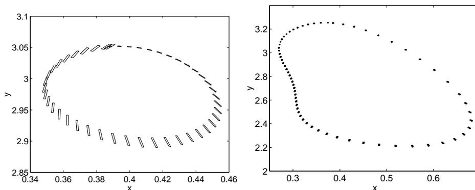
Figure 7.16: Periodic solution of the forced Brusselator, using the parameters  $A = \frac{2}{5}$ ,  $B = \frac{6}{5}$ ,  $a = .03$ , and  $\omega = \frac{\pi}{4}$ . The left figure shows the period  $p = 1$  solution, and the right figure shows the period  $p = 2$  solution.
