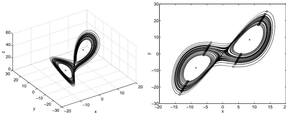
Figure 7.11: Floating-point solution of Eq. (7.5) using  $b = \frac{8}{3}$ ,  $r = 28$  and  $\sigma = 6$ . The left graph shows the result of the computations in a three-dimensional phase plot. In the right graph, a projection of the solution to the  $(x, y)$  plane is seen and the intersection of the solution with the plane  $z = 27$  has been marked with small circles. The stationary points have been marked with '+' on both figures.
