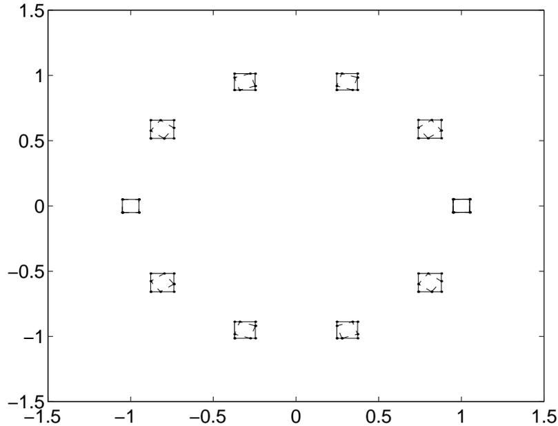
Figure 4.3: Ten interval iterations of the extended mean value enclosure of the map in Eq. (4.3) with  $\Delta t = \frac{\pi}{5}$  and the initial interval vector  $([x_0], [y_0]) = ([0.95, 1.05], [-0.05, 0.05])$ . The solid rectangles are the interval vector enclosures  $\{([x_j], [y_j])\}_{j=0, \dots, 10}$  while the dashed rectangles are the rotating rectangle enclosures  $\{A_{j+1}\hat{r} \mid \hat{r} \in [\hat{r}_{j+1}]\}$ , for  $j = 1, \dots, 10$ .
