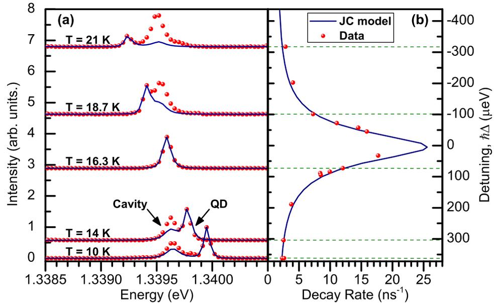
**Figure 3.** (a) The measured spectra (red circles) for a QD in a micropillar cavity for various values of the detuning that is controlled through the temperature  $T$ . The blue line is the corresponding theory without any free fitting parameters, as explained in the text. (b) Measured mean decay rate (red circles) as a function of detuning with a comparison to the theoretical predictions (blue line). These decay rate data have been published previously in [7].
