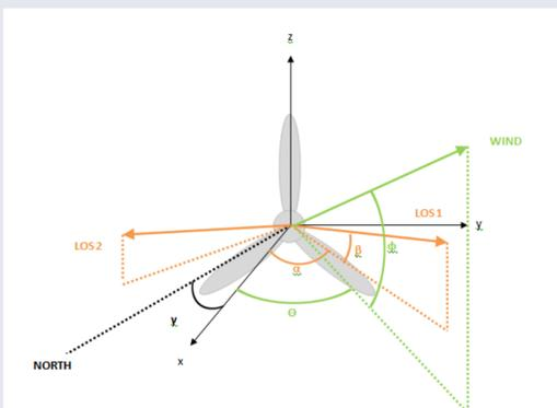
Sketch showing the lidar lines of sight and the wind vector. The x-axis is aligned with the lidar axis.  $\alpha$  is the beam half-opening angle;  $\beta$  the beam vertical angle;  $\theta$  the horizontal wind direction and  $\phi$  the vertical flow inclination
