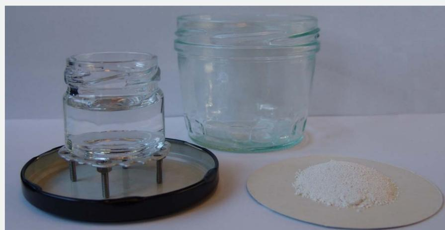
Figure 1. The unassembled migration cell. To the left is the metal screw cap, with a special designed rack on, and on top a small glass jar containing the saturated salt solution. To the right is a paperboard sample with MPPO on top. In the back is the glass jar.
