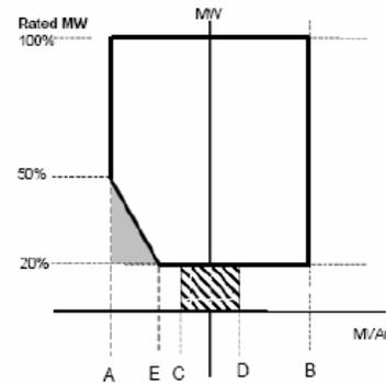
Point A is equivalent (in MVar) to: 0.95 leading Power Factor at Rated MW output
