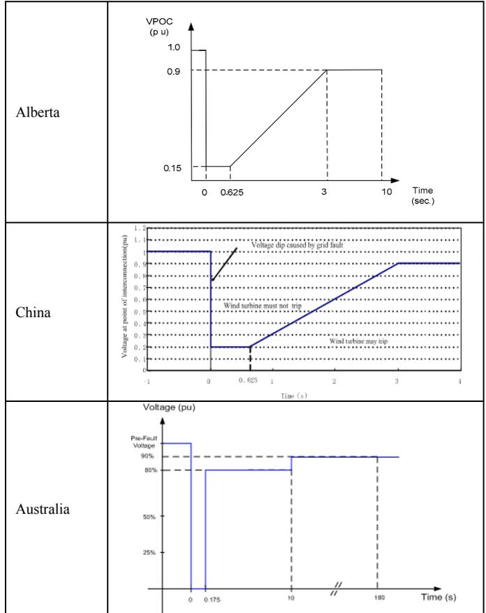
In order to deal with the LVRT requirements requested by TSOs, the wind turbine manufactures have specified the LVRT capability of their products. The LVRT capabilities of wind turbines from different manufactures may differ a little bit to each other. Basically, the LVRT capability of the wind turbines is to change the operation mode of the wind turbines under the specified low voltage conditions and stay connected if the WTG terminal voltage is within its defined low voltage conditions.
