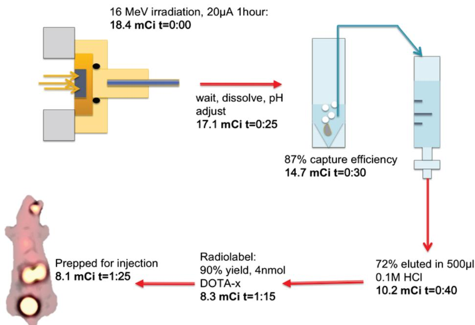
**FIGURE 2.** A graphical overview of the entire production procedure. The times listed are relative to EoB. The overall yield from start to finish is 24%, not decay corrected. The impurities in the 8.1mCi product are as follows:  $^{44m}\text{Sc}$  (63  $\mu\text{Ci}$ ),  $^{43}\text{Sc}$  (201  $\mu\text{Ci}$ ),  $^{48}\text{Sc}$  (103  $\mu\text{Ci}$ ) and  $^{47}\text{Sc}$  (27  $\mu\text{Ci}$ ).
