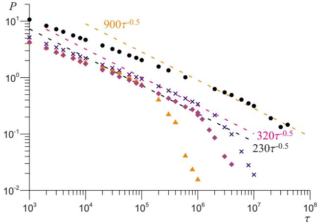
FIG. 3. (Color online) The average number of kinks versus quench time for the quadratic temperature dependence of the critical current  $f(t)=[1-T(t)/T_c]^2$ . The junction lengths are 2000, 1000, 800  $\lambda_J$  (from top to bottom). By triangles the number of kinks is shown for an annular junction of the length  $L=800$ .
