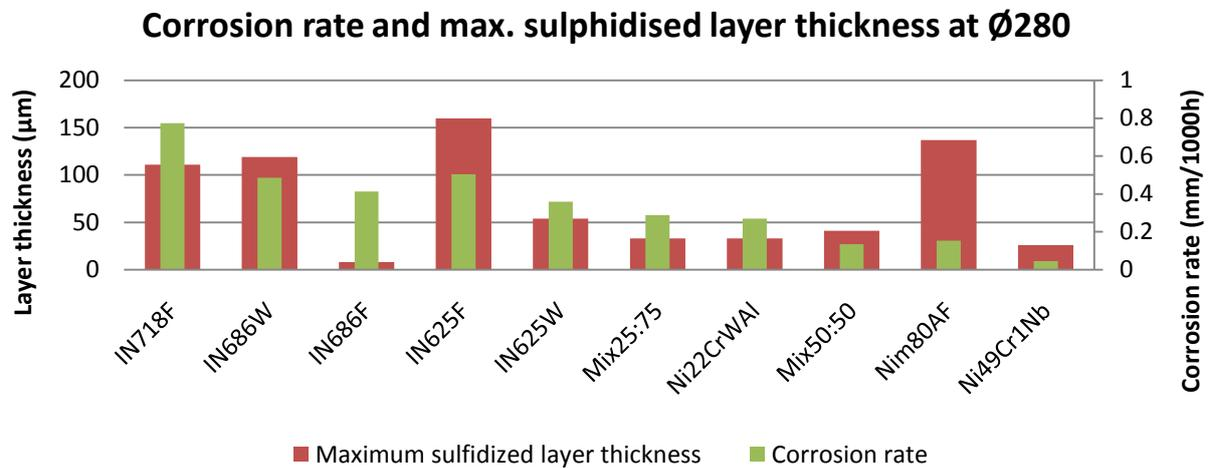
**Figure 6.** The corrosion rate measured over 2223 h of service time. The sulphidised layer for all HIP'd materials is moderate, while it for all others except IN686F is thicker. There does not seem to be any relation between the sulphidised layer thickness and the corrosion rate.
