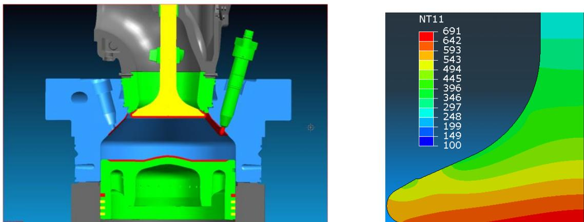
**Figure 2.** (Left) The hottest surfaces of the combustion chamber are marked with red. In this work the spindle bottom is treated. (Right) An FEM contour map of temperatures in °C. Because the cylinder is fitted with off-spec fuel injection valves, the spindle bottom temperature is increased to reflect a worst-case scenario.
