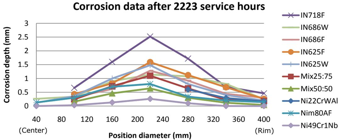
**Figure 3.** Corrosion depth compensated for the loss of Ni49Cr1Nb at same radial position.
