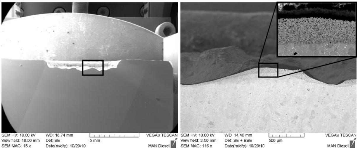
**Figure 4.** Cross section of IN625F material insert after 2223 hours of service. (Left) Overview. The surface has a wavy macro structure with peaks and valleys. This is found for all material inserts. (Right) Magnification of a peak. A sulphidized layer is found to be thickest at the peaks, but present throughout the surface, which is covered by an oxide layer of varying thickness.
