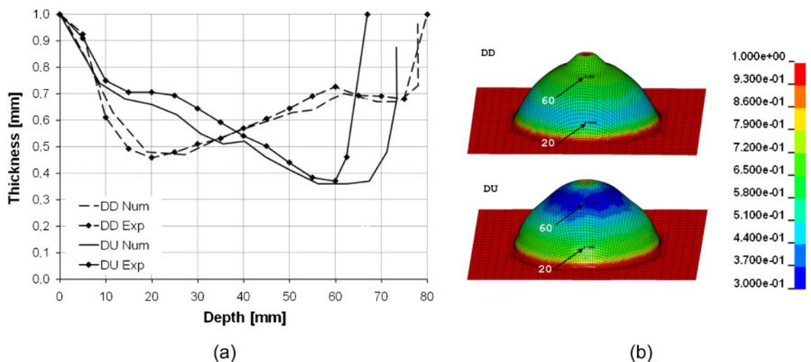
**Fig. 7** Second SPIF stage: (a) experimental and numerical evolution of thickness as functions of depth for DD and DU strategies; (b) final shapes for DD and DU strategies obtained from finite element modelling (scale in millimetres)
