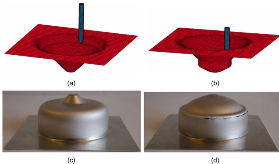
**Fig. 8** Multi-stage SPIF of a cylindrical cup: (a) formation of a plateau during the second stage (DD strategy) obtained from finite element modelling; (b) formation of a linear contact during the second stage (DU strategy) obtained from finite element modelling; (c) final part obtained from a multi-stage DDDU strategy; (d) final part obtained from a multi-stage DUD(D) strategy
