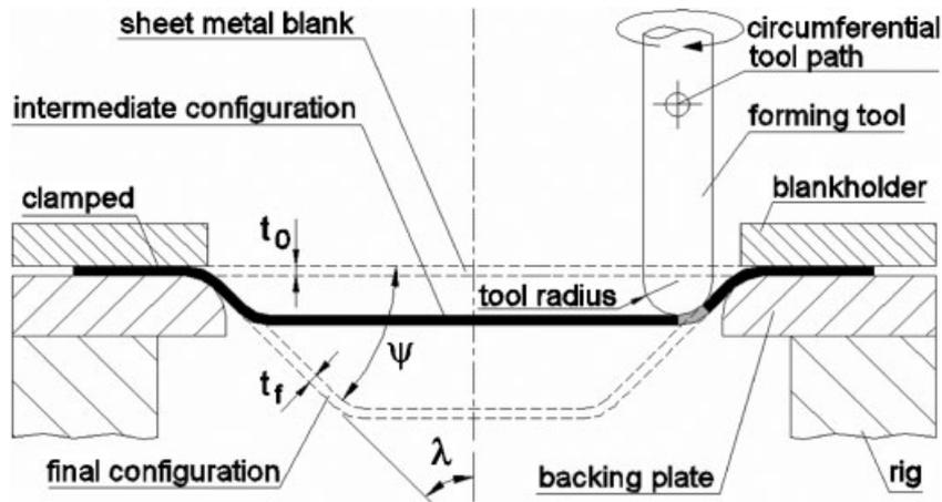
**Fig. 1** Schematic representation of a cross-sectional view of the rotational symmetric (SPIF) process
