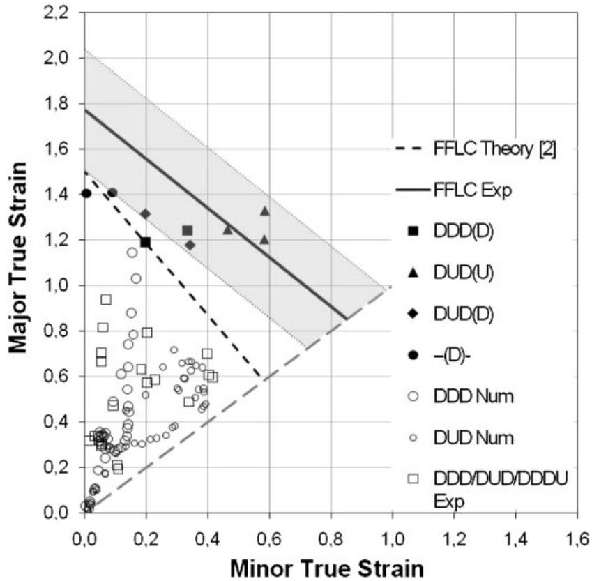
**Fig. 12** Fracture forming-limit diagram containing the FFLCs and the strain values obtained for different multi-stage SPIF strategies. Filled symbols indicate data measured at fracture locations whereas open symbols indicate data measured and computed along the meridional section slice in order to cover the whole geometry of the parts
