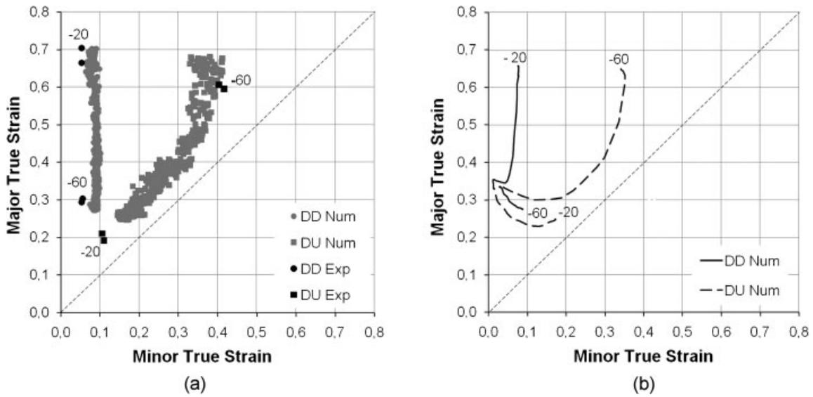
**Fig. 6** Second SPIF stage: (a) experimental and numerical strains for DD and DU multi-stage SPIF strategies, where the enclosed strain values are computed within the depth range 20–60 mm; (b) strain paths computed from two elements located within the depth range 20–60 mm
