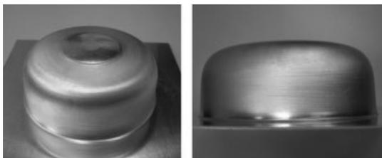
**Fig. 10** Cylindrical cup obtained by means of the enhanced multi-stage SPIF strategy
