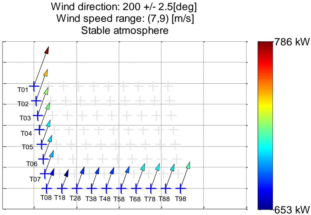
**Figure 1 – An example of power output variation along the south-western edge of Horns Rev 1 (the color and length of arrows is scaled with mean turbine power output, while their direction depicts wind direction in the considered flow case)**
