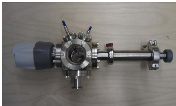
Figure 2. The ex situ INPS-TEM reactor. The system is shown with a TEM holder inserted, the pressure gauge and optical ports.
