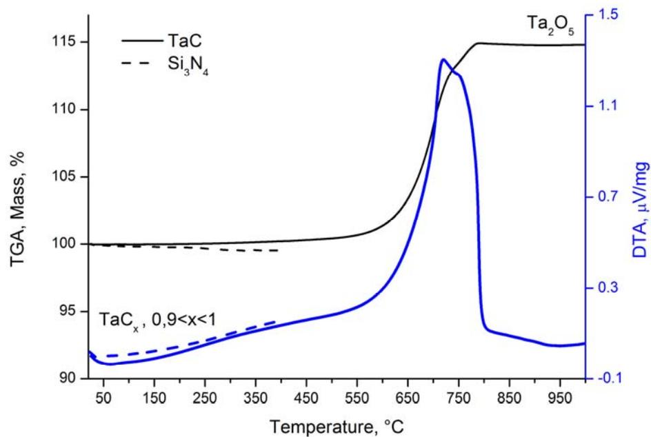
Figure 1. Thermogravimetric (thin line) and differential thermal analysis (thick line) curves of TaC and Si<sub>3</sub>N<sub>4</sub> in synthetic air. Heating rate 5 °C/min. Data for TaC is published as (2).
