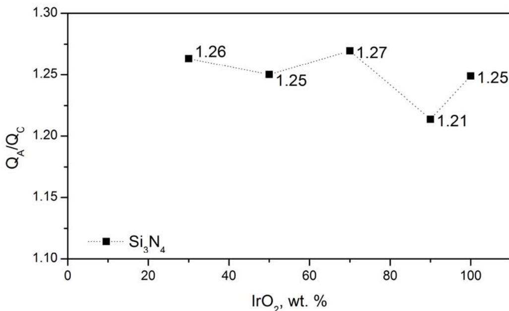
Figure 10. Ratio of anodic-to-cathodic charge for a IrO<sub>2</sub>/Si<sub>3</sub>N<sub>4</sub> supported electrocatalyst. Charge is integrated between 0.4 and 1.2 V. Potential sweep rate 500 mV/s, 0.5M H<sub>2</sub>SO<sub>4</sub>, room temperature.
