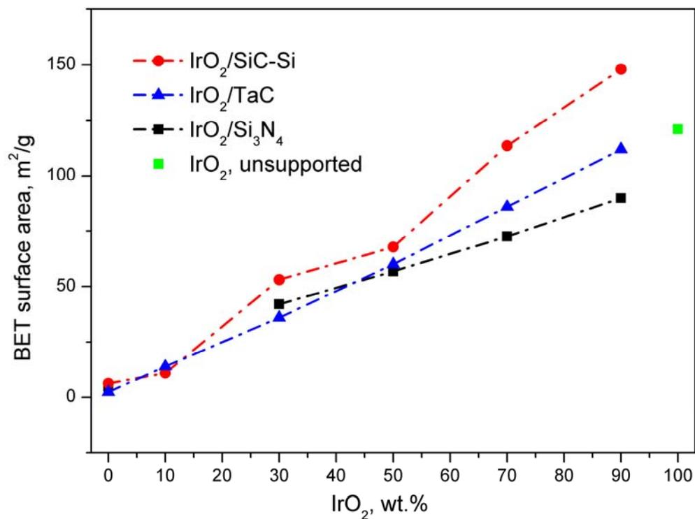
Figure 2. BET surface area of the prepared electrocatalysts. Data for IrO<sub>2</sub>/SiC-Si and IrO<sub>2</sub>/TaC is published as (1) and (2) respectively.
