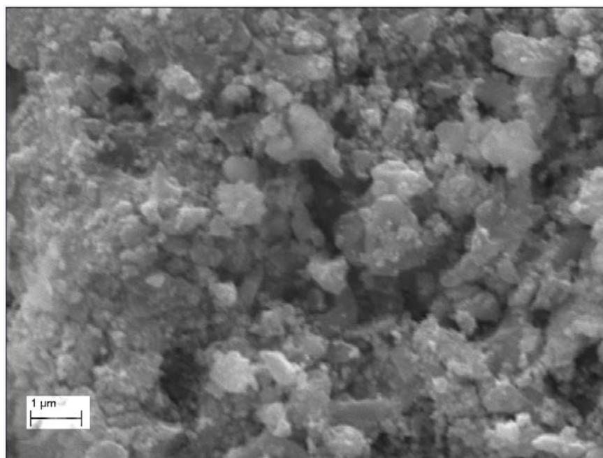
Figure 5. SEM image of 50 wt.% Si<sub>3</sub>N<sub>4</sub> electrocatalyst. Secondary electron detector used.
