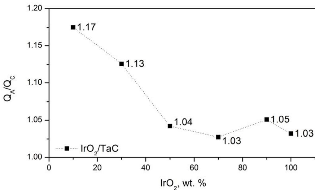
Figure 9. Ratio of anodic-to-cathodic charge for a  $\text{IrO}_2/\text{TaC}$  supported electrocatalyst. Charge is integrated between 0.4 and 1.2 V. Potential sweep rate 500 mV/s, 0.5M  $\text{H}_2\text{SO}_4$ , room temperature.
