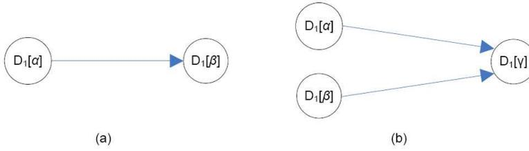
Figure 4.1: Graph representation of data flow: (a) for constraints of  $\alpha \subseteq \beta$ ,  $\alpha \setminus c \subseteq \beta$ , and  $\alpha \setminus (D) \subseteq \beta$ ; (b) for constraint  $\alpha \cap \beta \subseteq \gamma$ .
