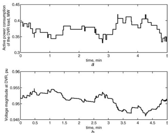
**Figure 5** DVR power consumption and voltage profile
