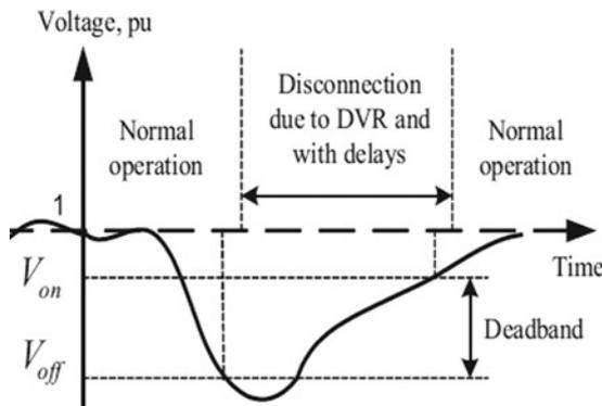
Figure 4 Illustration of DVR type I control
