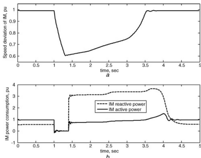
**Figure 2** Induction motor behaviour during voltage drop
