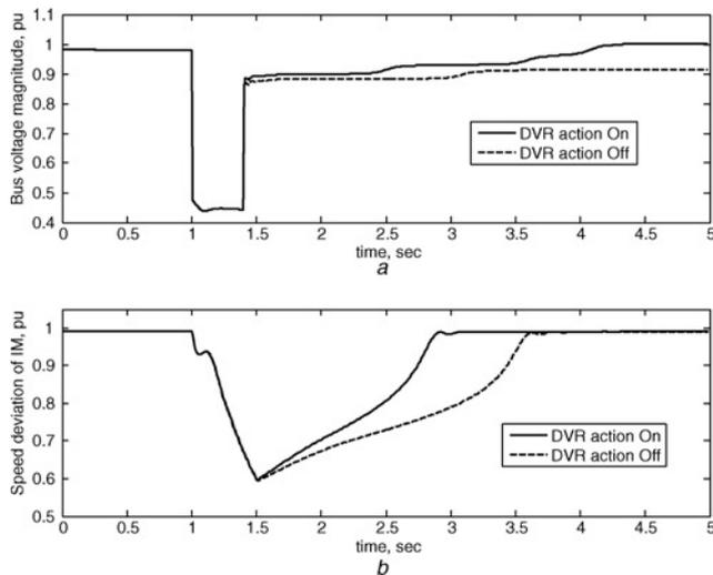
**Figure 7** Comparison analyses for on/off DVR performance
