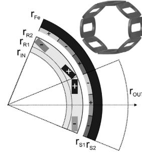
Fig. 3. Layout of 8 pole synchronous generator. The inner support structure spans from  $r_{in}$  and to the rotor between  $r_{R1}$  and  $r_{R2}$ . The stator windings of the 3-phases are spanned between  $r_{S1}$  and  $r_{S2}$ . An iron shield expands until  $r_{Fe}$  and the outer radius of the turbine nacelle is  $r_{out}$ . Inset: 3D representation of superconducting race-track rotor coils made of double pan-cake windings.
