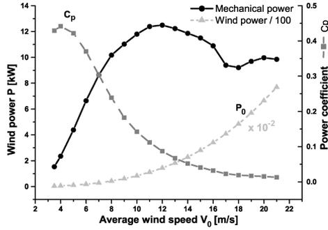
Fig. 1. Mechanical power curve  $P_{wind}$  of a small wind turbine as function the average wind speed when operated at a constant rotation speed of 56 rpm [2]. The wind power  $P_0 = (1/2)\rho v_0^3 A_{rotor}$  available at the rotor is scaled by a factor  $10^{-2}$  and is shown as well as the power coefficient  $C_P$  of the 2 blade rotor. A maximum of the available mechanical power  $P_{wind} = P_0 C_P$  of the rotor is seen at intermediate wind speed due to the stall limitation of  $C_P$ .
