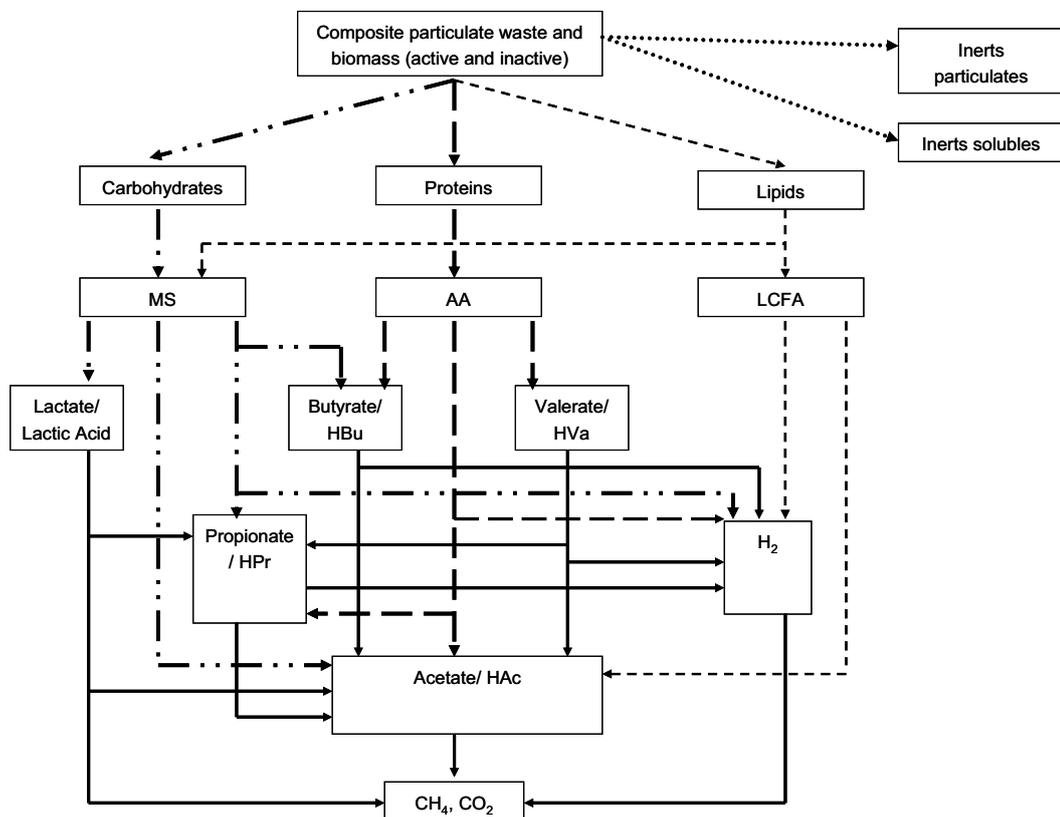
**Figure 3.** Organic fractions flow during anaerobic digestion. Dotted lines indicate flows regulated by the carbohydrates, proteins, and lipids available. Solid lines indicate flows regulated by the presence of intermediaries (volatile fatty acids, carbon dioxide, and hydrogen).
