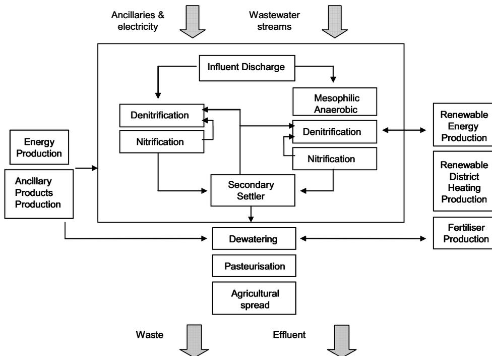
**Figure 14.** System boundaries of two biological treatment configurations. At the left is Denitrification/Nitrification plant, and at the right is Anaerobic pre-treatment followed by a Denitrification/Nitrification plant. The latter represents an alternative anaerobic pre-treatment unit in the production plant followed by the conventional treatment (V, VI).
