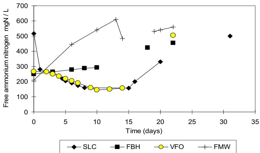
**Figure 7.** Free ammonium nitrogen for four of the wastewaters assessed by BMP assays during the first 35 days.
