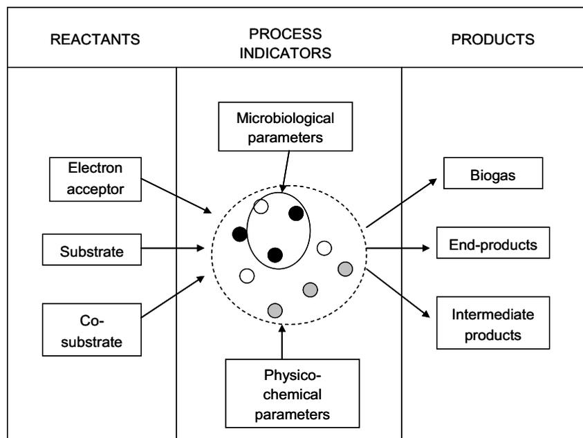
**Figure 4.** Parameters that can be assessed during a BMP assay. Adapted from *Rozzi and Remigi (2004)*.
