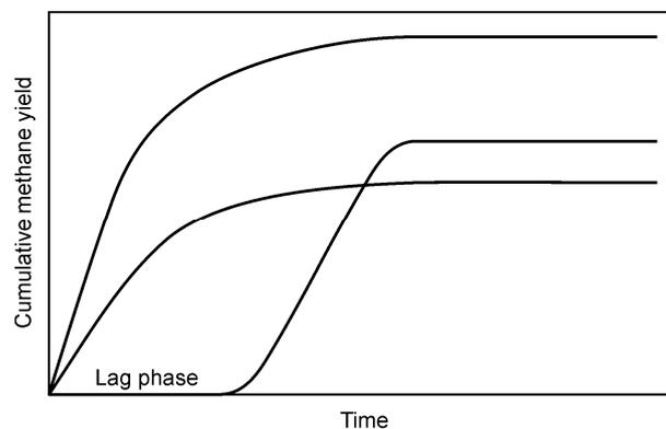
**Figure 2.** Typical cumulative methane production profiles during anaerobic batch degradation of organic waste(water)s.
