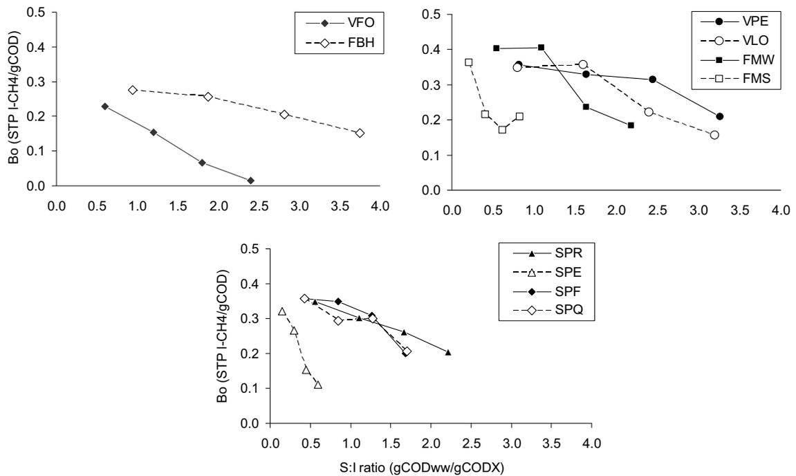
**Figure 5.** Influence of Substrate:Inoculum ratio on ultimate practical methane yield for wastewaters assessed at Paper I (adapted). For abbreviations see Table 1.
