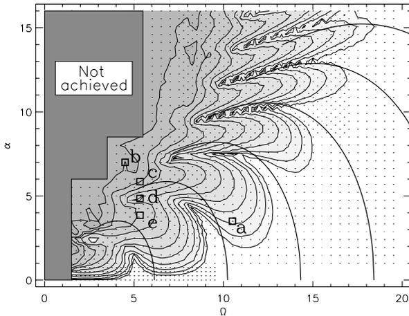
FIG. 4. Contour plot of the folding quantity  $F$  as a function of the control parameters  $\Omega$ ,  $\alpha$ . Points for each measurement of  $F$ ; squares for states shown in Fig. 2; solid curves for theoretical resonances predicted by Eq. (9).
