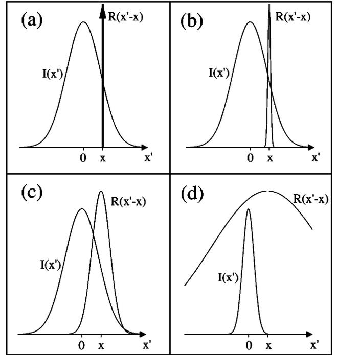
FIG. 1. Degrees of nonlocality, as given by the relative width of the response function  $R$  and the intensity profile  $I$  in the  $x$  plane. Shown is the local (a), the weakly nonlocal (b), the general (c), and the strongly nonlocal (d) response.
