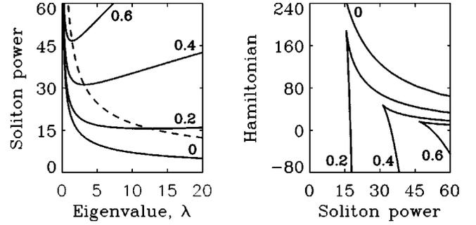
FIG. 3. 3D variational results with Gaussian response and trial function. Left: Soliton power (solid) versus eigenvalue  $\lambda$  for different degrees of nonlocality,  $\sigma=0, 0.2, 0.4$ , and  $0.6$ . Dashed lines show the threshold power (17). Right: Corresponding Hamiltonian versus power diagrams.
