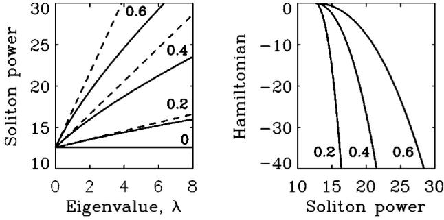
FIG. 2. 2D variational results with Gaussian response and trial function. Left: Soliton power (solid) versus eigenvalue  $\lambda$  for different degrees of nonlocality,  $\sigma=0, 0.2, 0.4$ , and  $0.6$ . Dashed lines show the weakly nonlocal approximation. Right: Corresponding Hamiltonian versus power diagrams.
