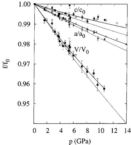
FIG. 4. Room-temperature ( $T_{\text{ref}}=300$  K) spinodal equation of state for experimental and theoretical data. Bold and empty symbols are the experimental data of Ming and Manghnani (Ref. 15) and Gerward *et al.* (Ref. 13), respectively. Solid lines represent the experimental SEOS fittings. Dashed lines were calculated from the theoretical SEOS fittings.
