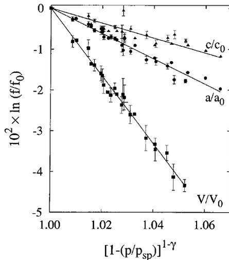
FIG. 2. Spinodal fitting to experimental data. Symbols represent the experimental data of Ming and Manghnani (Ref. 15) (with error bars) and Gerward *et al.* (Ref. 13) (without error bars). Solid lines represent the fitting functions [Eq. (5)].
