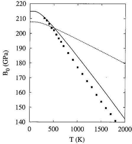
FIG. 6. Zero-pressure bulk modulus of rutile as a function of temperature. Symbols represent the experimental data of Saxena *et al.* (Ref. 17). The solid line is the thermal SEOS calculated from the  $(V/V_0 - p)$  experimental data at  $T_{\text{ref}} = 300$  K; the dashed line is the thermal SEOS calculated from the theoretical *aiPI*  $(V/V_0 - p)$  data.
