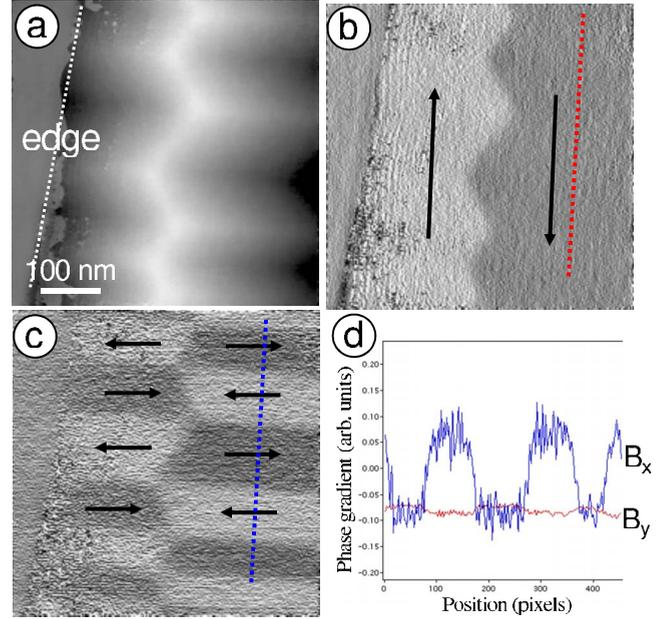
FIG. 3. (Color online) (a) Reconstructed electron-optical phase shift  $\varphi(x, y)$  from off-axis electron hologram. (b) and (c), the two phase gradient components, are proportional to the  $y$  and  $x$  components of the local magnetic induction within the sample. (d) Profiles of  $B_y$  and  $B_x$  components extracted from the phase gradient.
