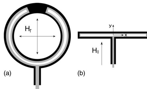
FIG. 1. (a) Gapped annular and (b) linear  $\delta$ -biased Josephson tunnel junctions. The base electrodes are in black, the top electrodes are in gray, and the junction areas are white. A gapped annular junction in a radially uniform magnetic field  $H_r$  is topologically equivalent to a linear junction in an in-plane uniform field  $H_{\parallel}$ .
