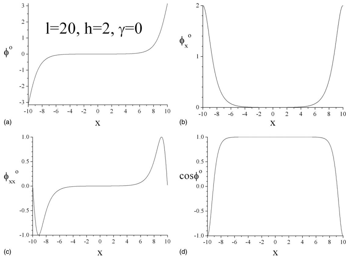
FIG. 4. (a) Phase profile  $\phi^o(x)$  as in Eq. (15) for  $\gamma=0, h=2$ , and  $l=20$ , (b) its first derivative, (c) its second derivative, and (d) its cosines. Note that  $\sin \phi^o(x) = \phi_x^o(x)$  and  $\cos \phi^o(x) = 1 - [\phi_x^o(x)]^2/2$ .
