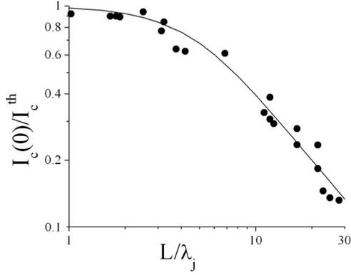
FIG. 8. Log-log plot of the measured zero-field critical currents  $i_c(0)$  of many  $\delta$ -biased JTJs versus their reduced length  $L/\lambda_j$ . The critical current has been normalized to the small junction theoretical value calculated as the 70% of the current jump at the junction gap voltage. The solid line is obtained from Eq. (11) with  $\gamma_c$  as in the empirical Eq. (12).
