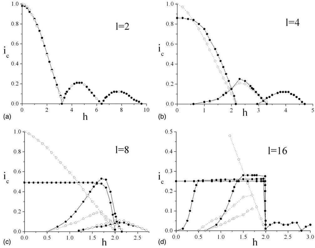
FIG. 6. Numerically computed magnetic diffraction patterns for different junction normalized lengths. From (a) to (d)  $i_c$  vs  $h$ , respectively, for  $l=2, 4, 8, 16$ . The full dots refer to point-injected bias current, while, for the sake of comparison, the open dots correspond to the well-known case of a uniformly biased junction.
