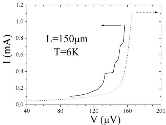
FIG. 11. Profiles of the first zero-field step for overlap junctions with  $L=150$   $\mu\text{m}$  and  $J_c=3$  kA/cm<sup>2</sup> (corresponding to  $\lambda_j \approx 12$   $\mu\text{m}$ ). (a)  $\delta$  bias (solid line) and (b) uniform bias (dashed line). The data were taken at  $T \approx 6$  K. The arrows indicate the switching direction at the top of the step.
