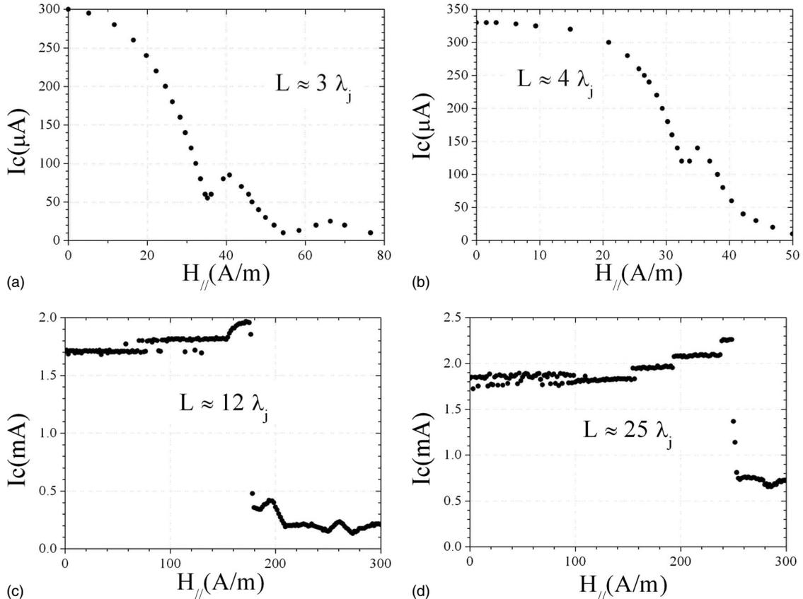
FIG. 9. Experimental magnetic diffraction patterns taken for linear samples in a uniform in-plane field with increasing normalized lengths  $l=L/\lambda_j$ . (a)  $L=250 \mu\text{m}$  and  $\lambda_j \approx 80 \mu\text{m}$ , (b)  $L=300 \mu\text{m}$  and  $\lambda_j \approx 80 \mu\text{m}$ , (c)  $L=150 \mu\text{m}$  and  $\lambda_j \approx 12 \mu\text{m}$ , and (d)  $L=300 \mu\text{m}$  and  $\lambda_j \approx 12 \mu\text{m}$ .
