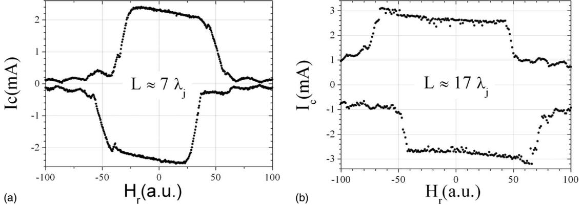
FIG. 10. Experimental magnetic diffraction patterns in a radially uniform magnetic field  $H_r$  for two gapped annular samples having the same critical current density  $J_c=3$  kA/cm<sup>2</sup> (corresponding to  $\lambda_j \approx 12$   $\mu\text{m}$ ) and different lengths  $L$ . (a)  $L=82$   $\mu\text{m}$  and (b)  $L=200$   $\mu\text{m}$ .
