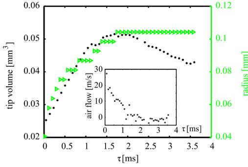
FIG. 5 (color online). Measured minimal neck radius (triangles) and tip volume (filled circles) as functions of time to pinch-off for  $R_{\text{drain}} = 1.2$  mm and  $\Omega = 13.5$  rpm. The compressibility of the air in the tip is negligible, since once the neck reaches the resolution of our recordings ( $1 \mu\text{m}$ ) the air is found to be compressed less than 1%. The average flow velocity through the collapsing neck (inset) is therefore computed directly from the volume change.
