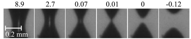
FIG. 2. Bubble pinch-off at the tip of the bathtub vortex for  $R_{\text{drain}} = 1.2$  mm and  $\Omega = 13.5$  rpm. The time to pinch-off in milliseconds is shown above each frame. Note that the axial downflow around the tip does not give rise to any apparent up-down asymmetry in the pinch-off region, and that we observe a symmetric pinch-off as expected for bubble formation.
