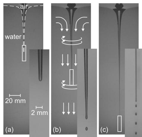
FIG. 1. By increasing the rotation rate while keeping  $R_{\text{drain}} = 1.2 \text{ mm}$ , the air-filled tip of the bathtub vortex goes from a stable state at 13.5 rpm (a) to an unstable bubbling state at 24 rpm (b) and 30.5 rpm (c). In the bubbling state the frequency of bubble formation increases and the bubble size decreases with increasing rotation rate as shown in (b) and (c) for typical cases.
