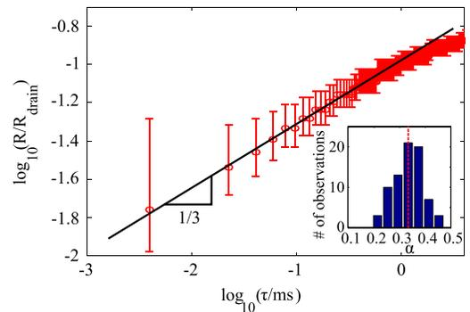
FIG. 3 (color online). Measured radius of the air-filled neck as a function of the time to pinch-off (circles) and power law with exponent  $\alpha = 1/3$  (solid line).  $R_{\text{drain}}$  is 1.0 mm and  $\Omega$  is 42 rpm. Inset: Frequency histogram for the measured exponents with  $\alpha = 1/3$  indicated.
