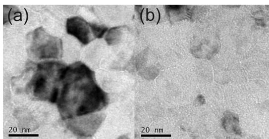
FIG. 5. Underfocused (bright-field) TEM images of the samples deposited at biases of (a)  $-150$  V and (b)  $-200$  V. The picture in (b) shows a large quantity of tiny white dots, which are interpreted as small Ar bubbles.
