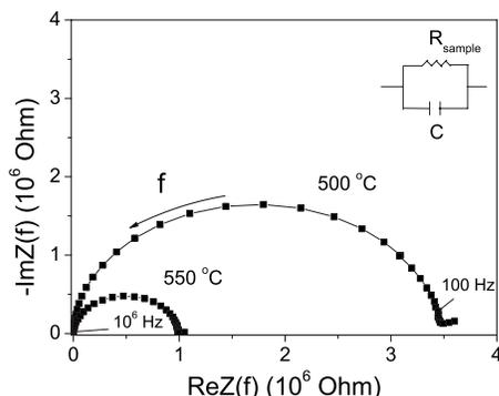
FIG. 7. Typical impedance spectra measured at 500 and 550 °C for a film with thickness  $d=1 \mu\text{m}$  deposited on quartz at 400 °C with a bias of  $-70 \text{ V}$ . The frequency range used was 1 MHz–42 Hz.
